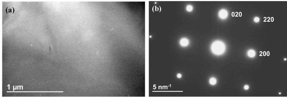
Fig. 2. TEM confirmation of the single-phase  $\gamma$ -structure of designed alloy. (a) Dark-field image. (b) Selected area electron diffraction pattern.
