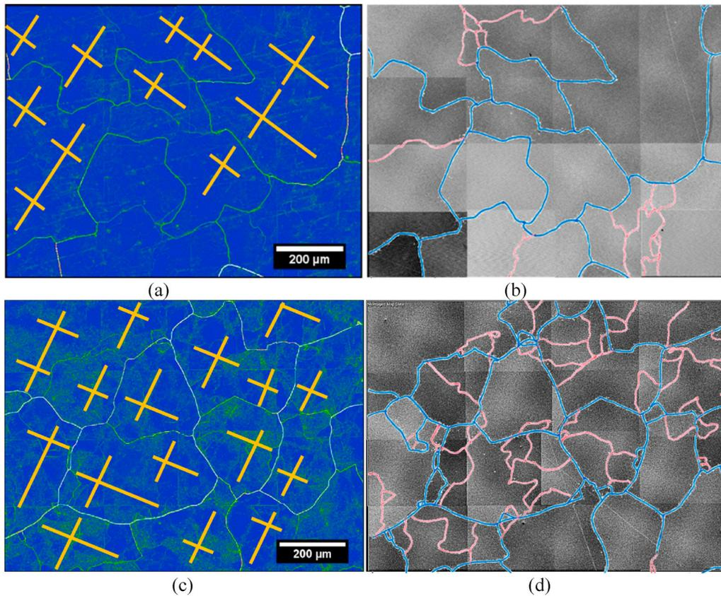
**Fig. 9.** Comparison of the subgrain structure of [001] specimens of  $\gamma$ -alloy before (a, b) and after (c, d) creep at 1288 °C, 10 MPa and 7 % creep strain. EBSD analysis with KAM mapping (a,c) and scattered electrons images (b,d). See text for details.
