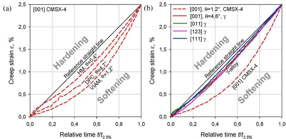
Fig. 6. Creep strain vs. normalized time  $t/t_{2.5\%}$ , 1288 °C, and 10 MPa. (a) [001] CMSX-4 crystals from different producers, VIAM, DPC, and HM. The deviations  $\theta$  from the [001] ideal orientation are given in the graph. (b) Comparison between the  $\gamma$ -alloy and CMSX-4. The solid lines correspond to  $\gamma$ -alloy crystals of different orientations, the dashed line to a [001] CMSX-4 specimen.
