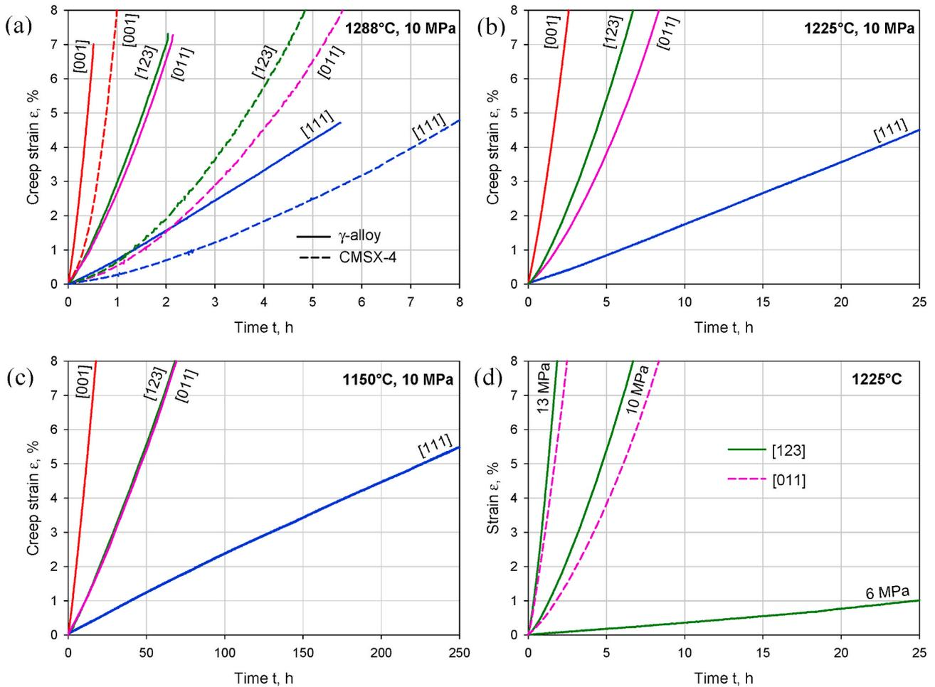
Fig. 5. Creep curves of  $\gamma$ -alloy single-crystals of different orientations at 1288 °C (a), 1225 °C (b, d), and 1150 °C (c). (a–c) Different temperatures but the same stress of 10 MPa. (d) Temperature of 1225 °C but different stresses, 6, 10, and 13 MPa. (a) Comparison of  $\gamma$ -alloy with CMSX-4 at 1288 °C and 10 MPa.
