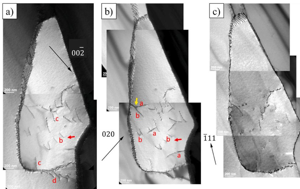
**Fig. 11.** Dislocations inside a subgrain in the necking area of a [001] specimen ruptured during a creep test at 1288 °C and 10 MPa. The overall creep strain is 33 % and the estimated local strain is 55 %. Bright field two-beam TEM micrographs, the diffraction vector is indicated.
