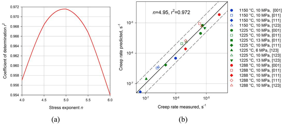
**Fig. 12.** Joint fitting of the creep results considering the measured specimen orientations ( $\theta, \rho$ ). (a) Variation of the coefficient of determination  $r^2$  with  $n$ . (b) Comparison between measured and predicted creep rates.**Table 3**
