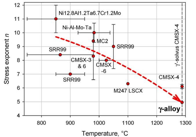
**Fig. 13.** Stress exponent  $n$  measured for superalloys at different temperatures (this work, [7,27]). Vertical and horizontal bars show respectively the scatter of  $n$  and the investigated temperature ranges. The dashed line shows the decreasing tendency of  $n$  with temperature.
