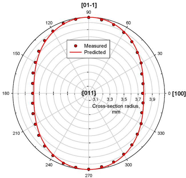
Fig. 8. Shape of the cross-section of a [011] specimen of the  $\gamma$ -alloy tested at 1288 °C, 10 MPa. The test has been interrupted at the creep strain of 7.3 %. The red dots and the elliptical red curve are respectively the experimental results and the theoretical prediction assuming {011}{111} octahedral slip. (For interpretation of the references to colour in this figure legend, the reader is referred to the Web version of this article.)
