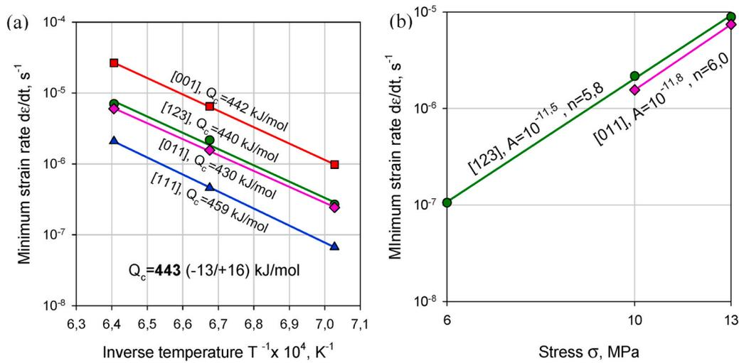
Fig. 7. Evaluation of the creep activation energy  $Q_c$  and the stress exponent  $n$  of the  $\gamma$ -alloy by the separated fitting of different orientations. (a) Fitting of  $Q_c$  for the creep tests at 1150 °C, 1225 °C, 1288 °C and the stress level 10 MPa. (b) Fitting of  $n$  for the creep tests at 1225 °C and stresses 6, 10, and 13 MPa.
