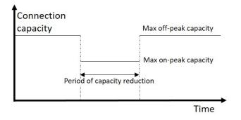
Figure 4: Example of variable capacity contract. Adapted from [87]
