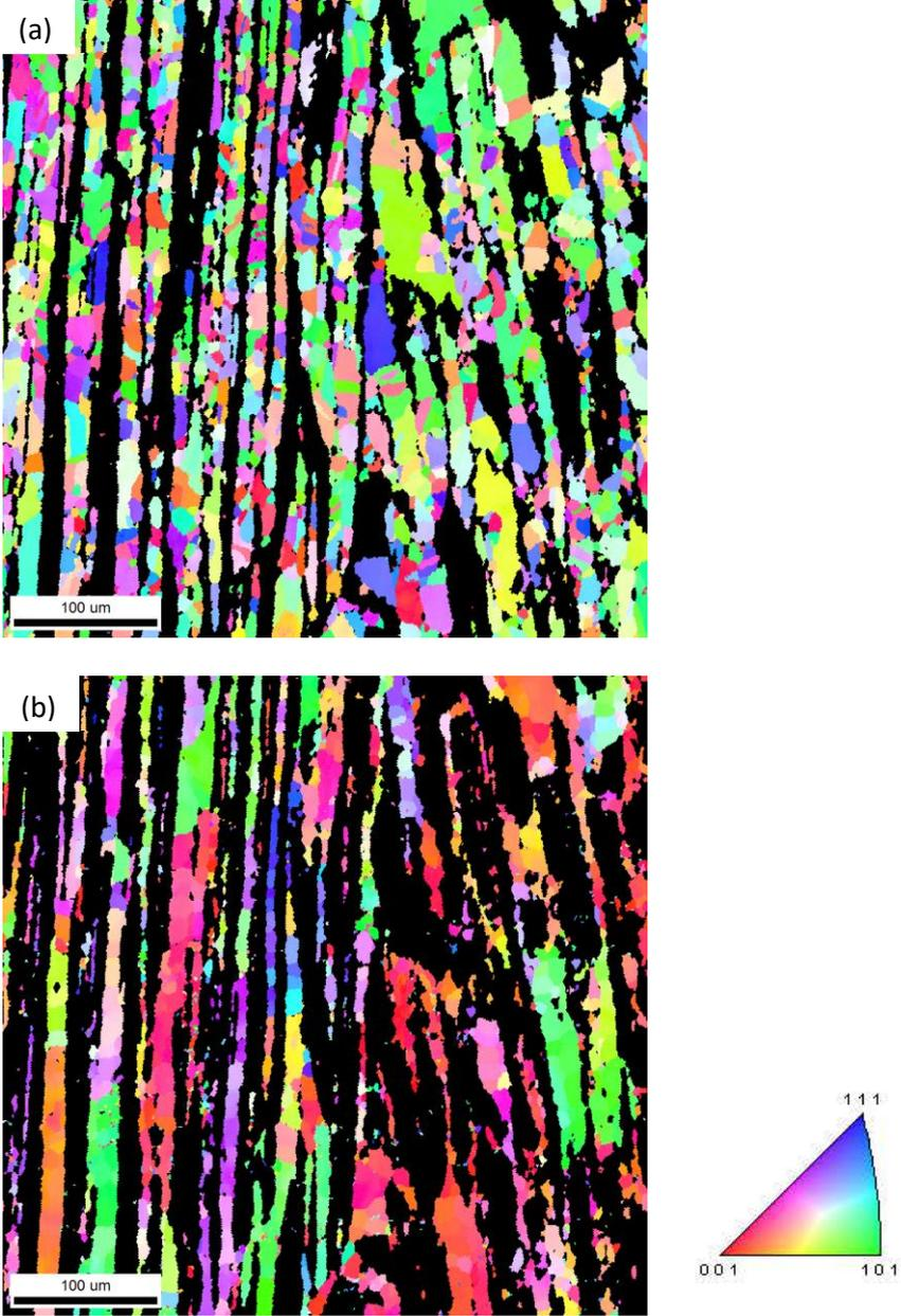
**Fig. 2.** EBSD orientation maps measured at the as received state, a) austenite, b) ferrite.
