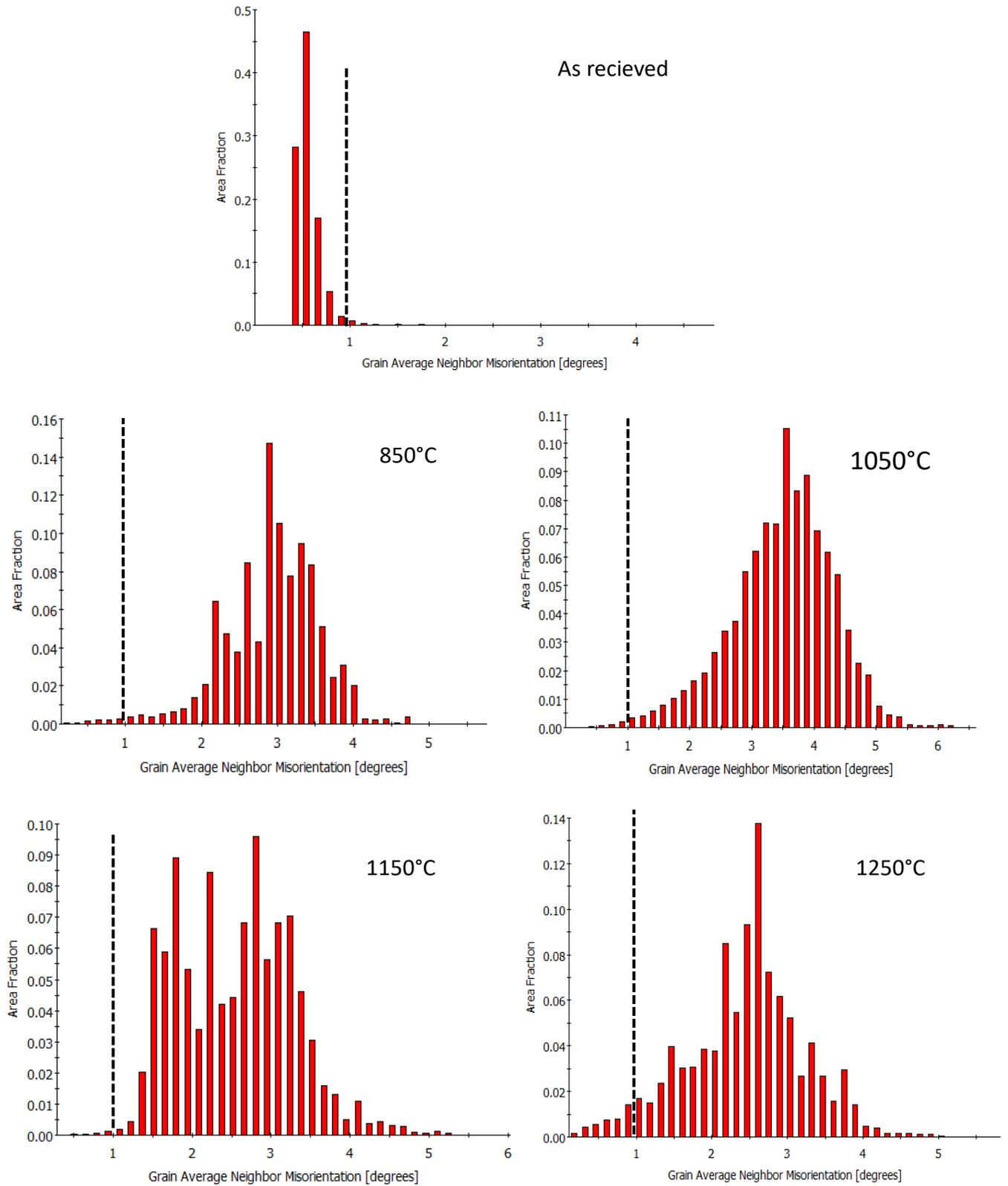
**Fig. 6.** GAM profiles assessed for the austenite phase in the as received state and after hot forging at various temperatures. The black dashed line indicates the difference between recrystallized from deformed grains.
