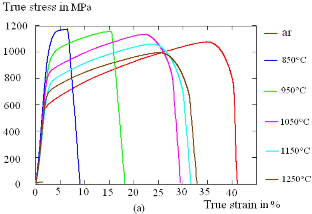
**Fig 11.** True stress-true strain curves after different forging temperatures.
