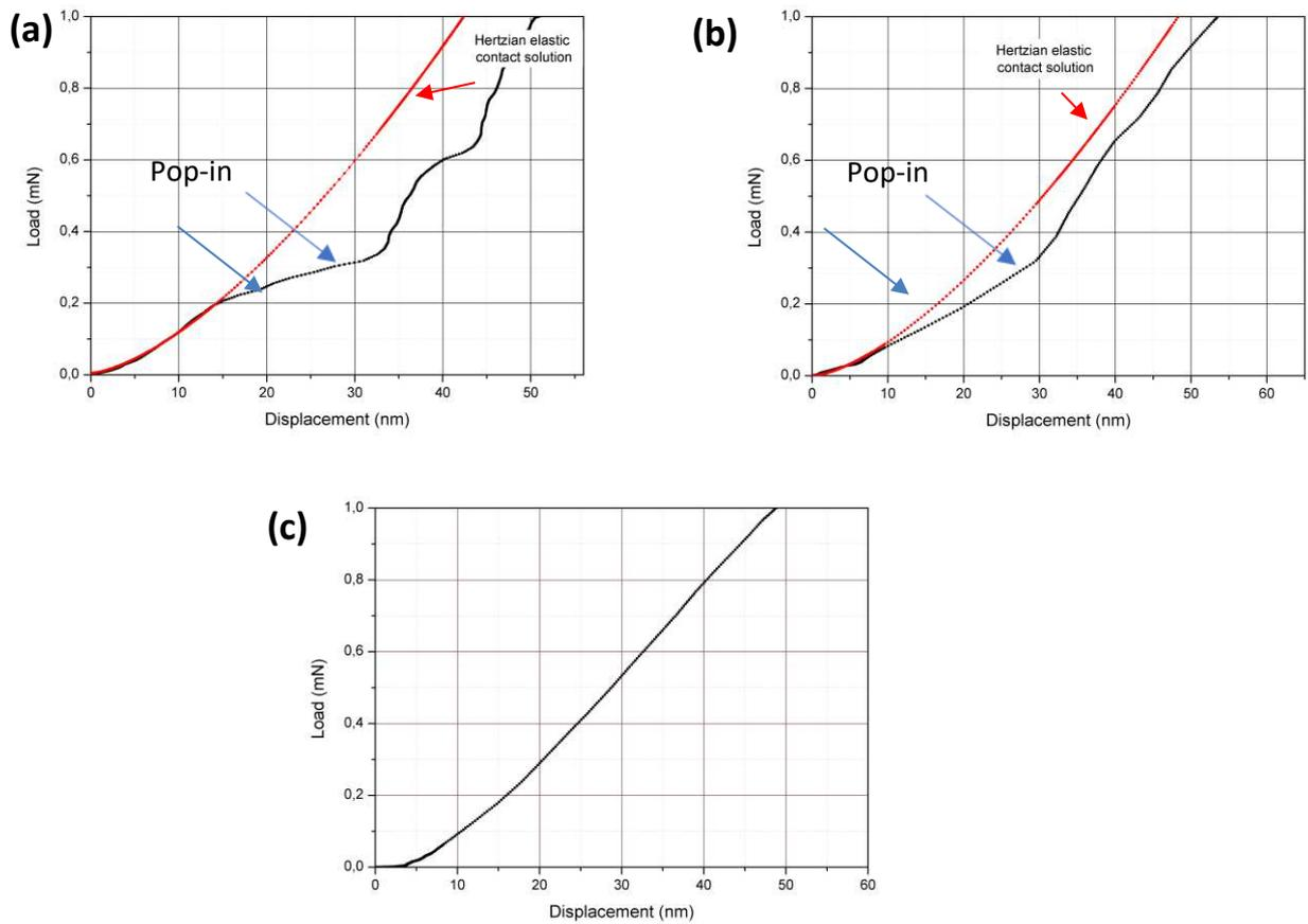
**Fig. 13:** Zoom view of loading segment of P-h curves of Fig. 12b including Hertzian elastic contact solution for (a): as-received state, (b) and (c): those obtained after 4 passes hot forging at 850°C 1250°C respectively.
