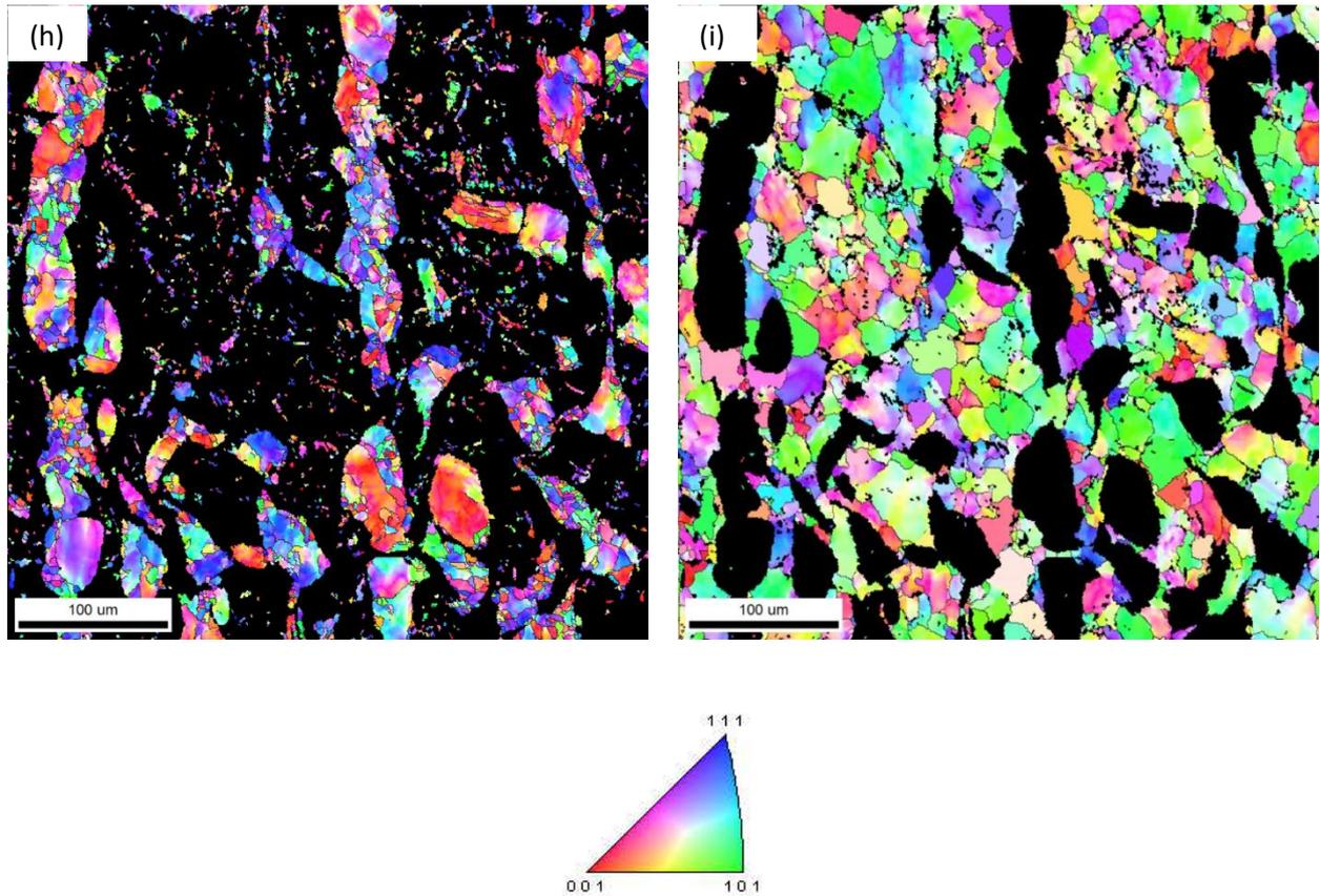
**Fig. 5.** EBSD orientation maps after 4 passes hot forging for respectively: (a), (b) and (c) austenite, ferrite and sigma phase at 850°C, (d) and (e) austenite and ferrite at 1050°C, (f) and (g) austenite and ferrite at 1150°C, (h) and (i) austenite and ferrite at 1150°C.
