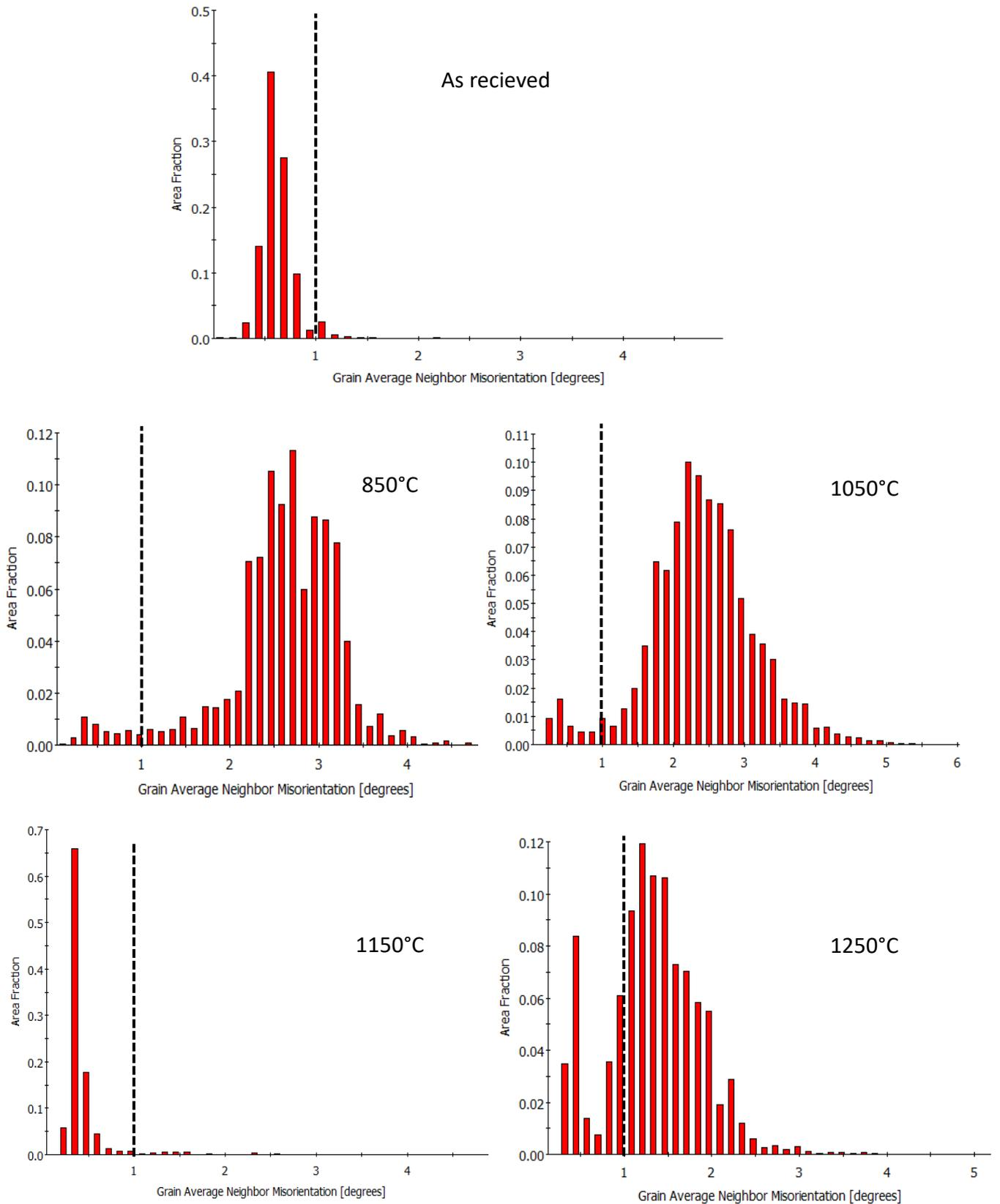
**Fig. 7.** GAM profiles assessed for the ferrite phase in the as received state and after hot forging at various temperatures. The black dashed line indicates the difference between recrystallized from deformed grains.
