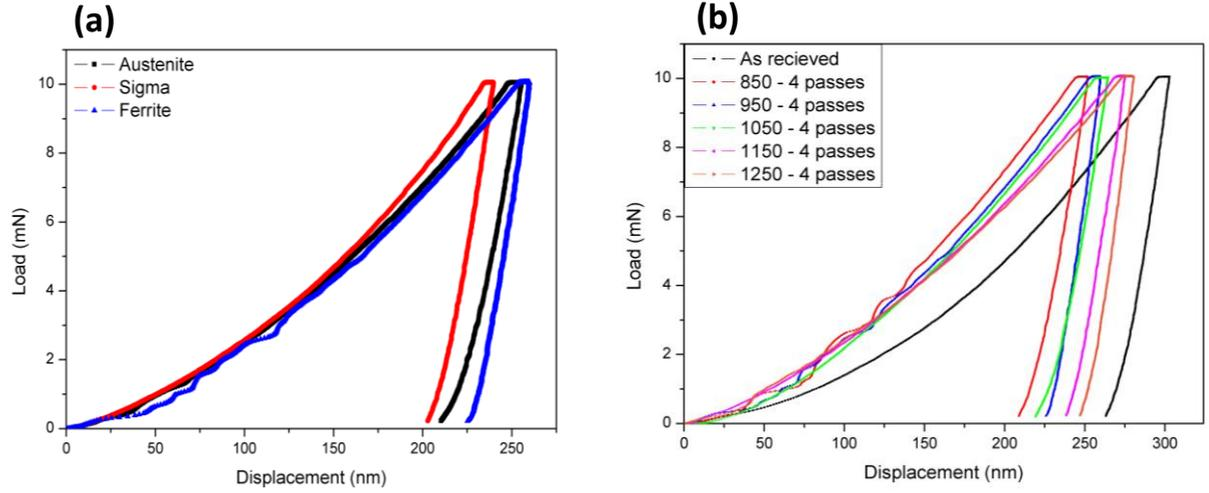
**Fig. 12:** Nanoindentation load-displacement curves of samples obtained after 4 passes hot forging : (a) – P-h curves of different phases (ferrite, austenite and sigma phase) at 850° (b) – Conducted in ferrite phase of samples at different temperatures.
