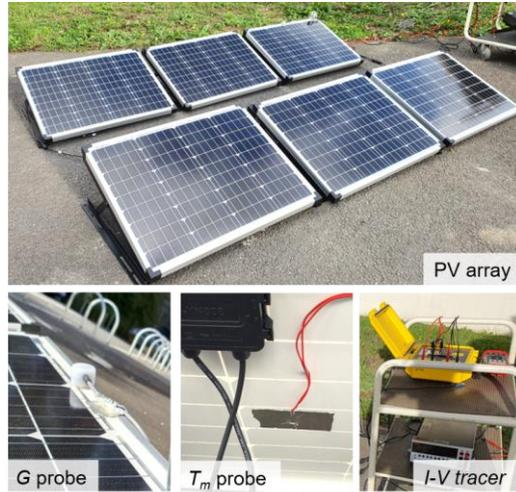
Fig. 13 Field test setup
