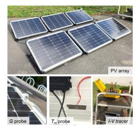
Fig. 13 Field test setup
