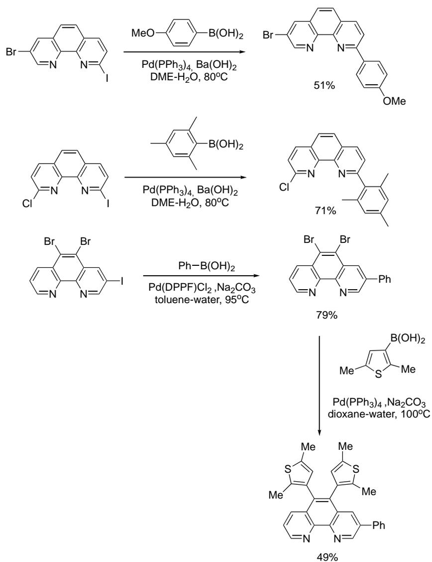
**Scheme 11.** Regioselective Pd-catalyzed Suzuki-Miyaura reaction of iodo-substituted Phens.
