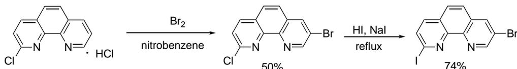
**Scheme 8.** Synthetic approach to 2-chloro- and 2-iodosubstituted 3-bromo-1,10-phenanthrolines.
