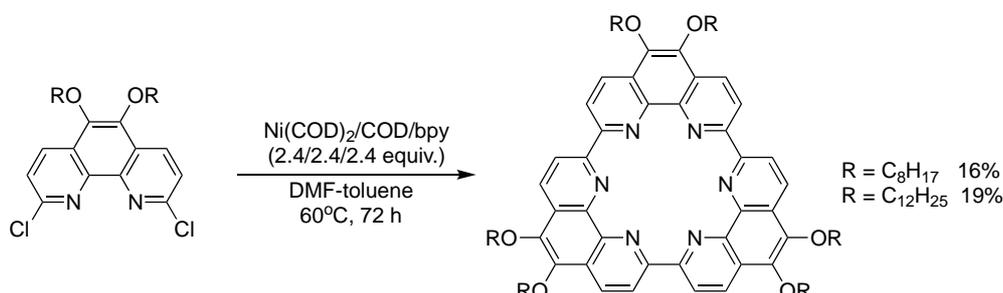
**Scheme 19.** Synthesis of the macrocyclic ligand *via* the reductive trimerization of 2,9-dichloro-1,10-phenanthroline derivatives.
