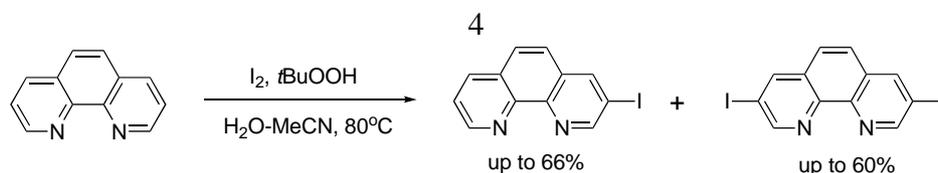
**Scheme 4.** Synthesis of 3-iodo- and 3,8-diiodo-1,10-phenanthrolines.
