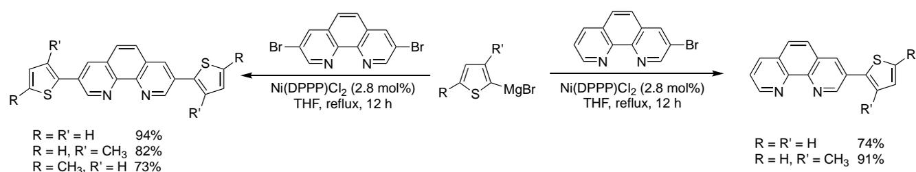
**Scheme 17.** Functionalization of Phens via the Kumada reaction.
