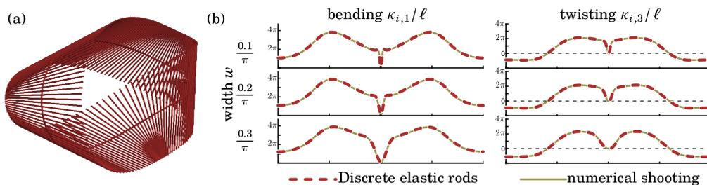
**Figure 5.4.** Simulation of an inextensible Möbius strip with  $L = 1$ . (a) Equilibrium width  $w = 1/(2\pi)$ , as simulated by the Discrete elastic rod model from Section 4(b) with  $N = 150$  nodes. (b) Distribution of bending and twisting: Discrete elastic rod simulations with  $N = 250$  vertices (dashed curves) versus solution of [14] obtained by numerical shooting (solid curves); the latter have been properly rescaled to reflect our conventions.
