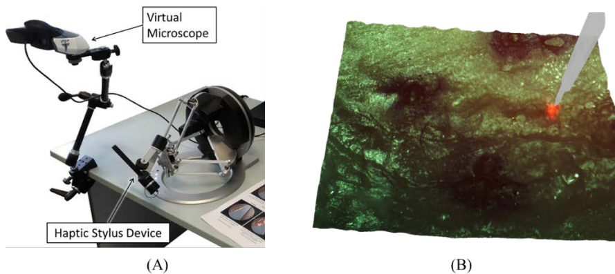
472 Fig. 16. The Haptic Laser Scalpel, developed to bring the sense of haptics to contactless laser surgeries. (A) Surgeon interface. (B) 3D 473 visualization of the surgical site with an augmented reality haptic scalpel avatar.
