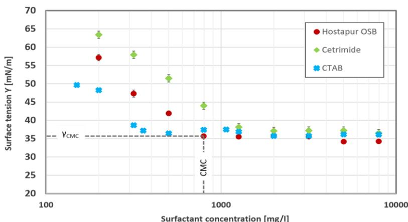
Figure 4: CMC evaluation of the three tested surfactants.
