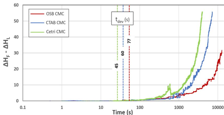
Figure 7: Evolution of  $\Delta H_F - \Delta H_L$  in time for Hostapur OSB, CTAB and Cetrimide at CMC.  $\Delta H_F - \Delta H_L$ : the difference between the foam height and the liquid height from  $t_0$ .
