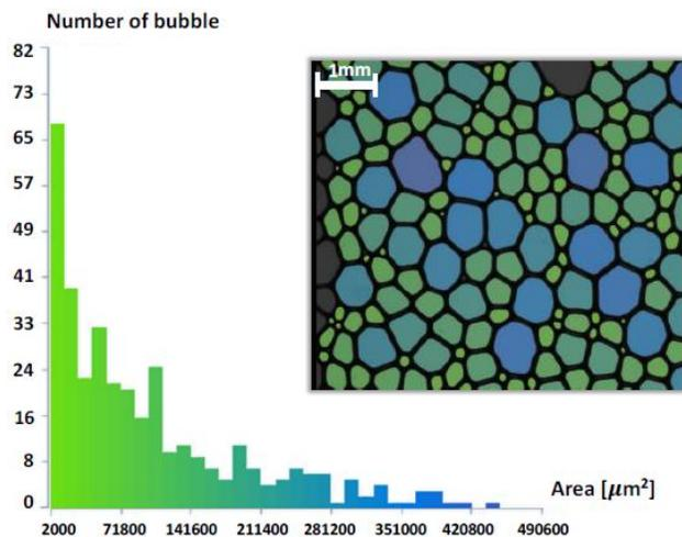
Figure 3: Bubble number distribution as a function of the area  $\mu\text{m}^2$  for the Hostapur OSB foam, produced with a concentration equal to the CMC, recorded 10 min after the end of foaming.
