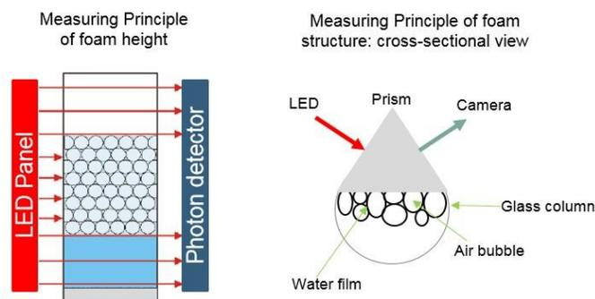
Figure 2: Concept of foam height and structure measurements [24]
