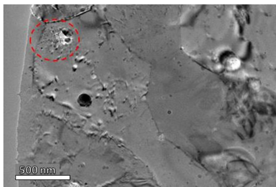
Figure 7: TEM bright field of sample 0.5P-I2 showing a cluster of particles due to an insufficient milling
