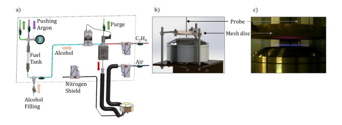
Figure 1: Experimental setup: a) Burner alimentation; b) 3D view of the burner with sampling probe and ceramic mesh disc; c) Picture of the flame on the McKenna burner.
