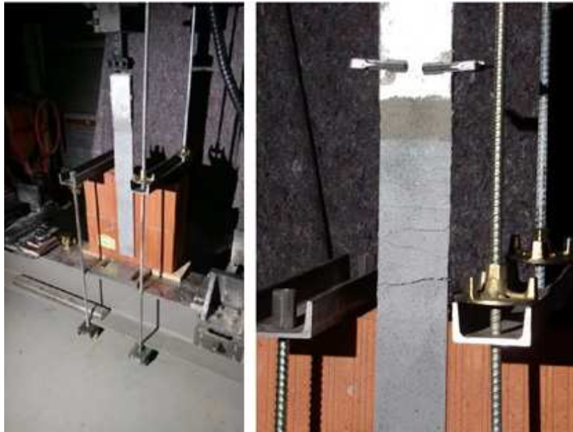
182 Figure 1: Test configuration for the SSGRM composite and development of the crack pattern 183 in the specimen.
