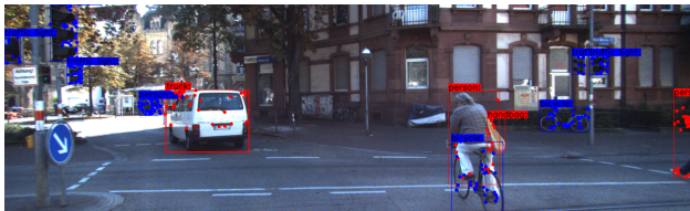
2.(d) Render the moving bounding box in red when the proportion of pixel-level outliers in the bounding box is over the threshold of 0.6
