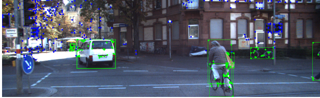
2.(b) Extract the Shi-Tomasi corner feature points, rendering in green for movable objects, rendering in blue for non-movable objects and background points
