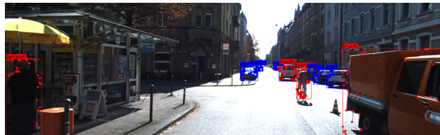
Fig. 5. Flow vector bound constraint for detecting moving objects with degenerate motion with the frame from KITTI raw data sequence 05
