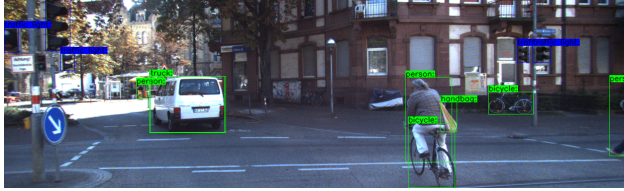
2.(a) Get the bounding boxes with semantic labels using yolo v4 detector
