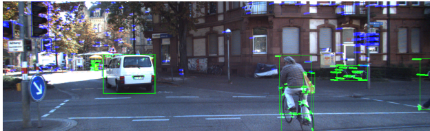
2.(c) Estimate the Fundamental matrix with the feature correspondences rendering in blue (pyramidal Kanade-Lucas-Tomasi tracker)
