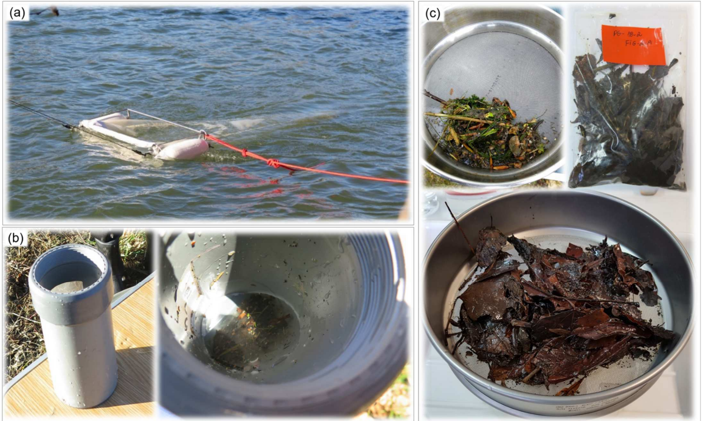
89 90 Figure 2. Sample collection in the field with (a) Manta trawl equipped with (b) a removal cod-end. Samples are filtered in the field (c) 91 using a 500 \mu\text{m} sieve and stored in a plastic bag before processing in the laboratory.
