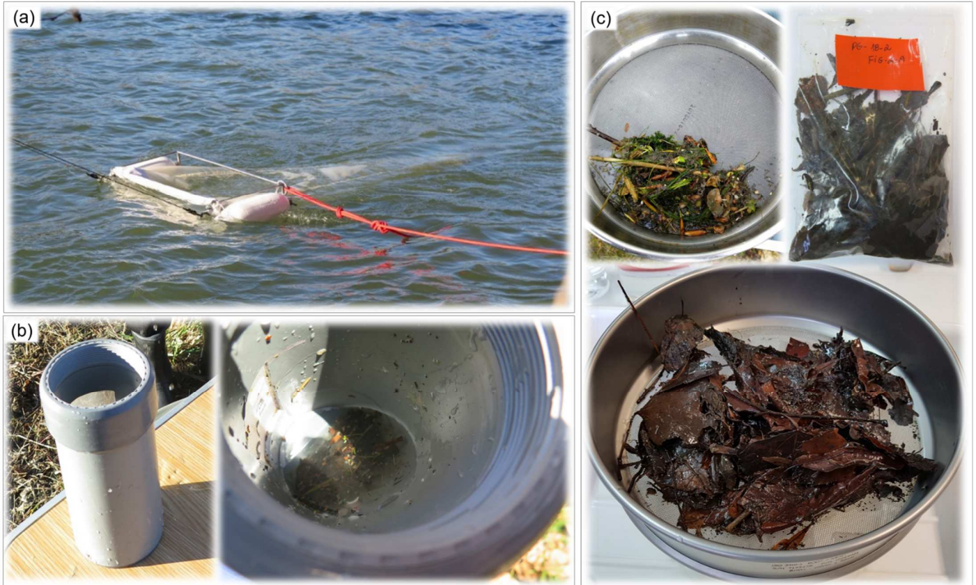
89 90 Figure 2. Sample collection in the field with (a) Manta trawl equipped with (b) a removal cod-end. Samples are filtered in the field (c) 91 using a 500 µm sieve and stored in a plastic bag before processing in the laboratory.
