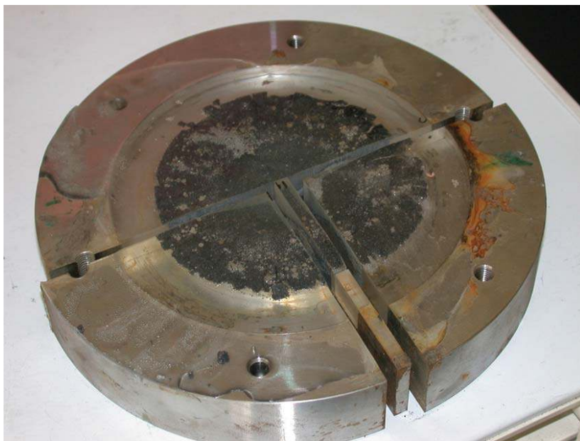
Figure 9.13. General macroscopic view of the recovered target and saw cut for further preparation of polished cross-section (see Figure 9.14)
