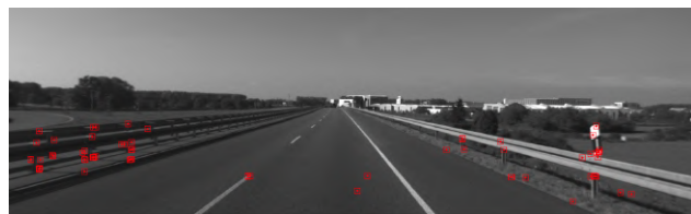
Fig. 5. Few distinctive ORB visual features for tracking on the highway scenario, KITTI sequence 01
