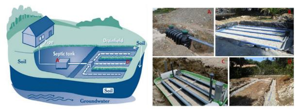
Fig. 1. Schematic representation of a septic system (adapted from EPA (2005)) and illustrative photos before filling operation (© KD, A: septic tank, B: sand filter, C: media filter, D: drain field).
