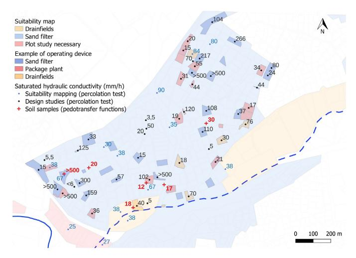
Fig. 4. Application of a soil-based methodology to the Montpellier case study. Source: Montpellier inter-municipality for suitability map, device in operation and measured permeability (black and blue numbers in millimeter per hour correspond to data from suitability mapping and design studies, respectively).
