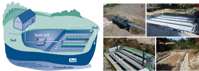
Figure 1: Schematic representation of a septic system (adapted from [45]) and illustrative photos before filling operation (© KD, A : septic tank, B : sand filter, C : media filter, D : drain field).
