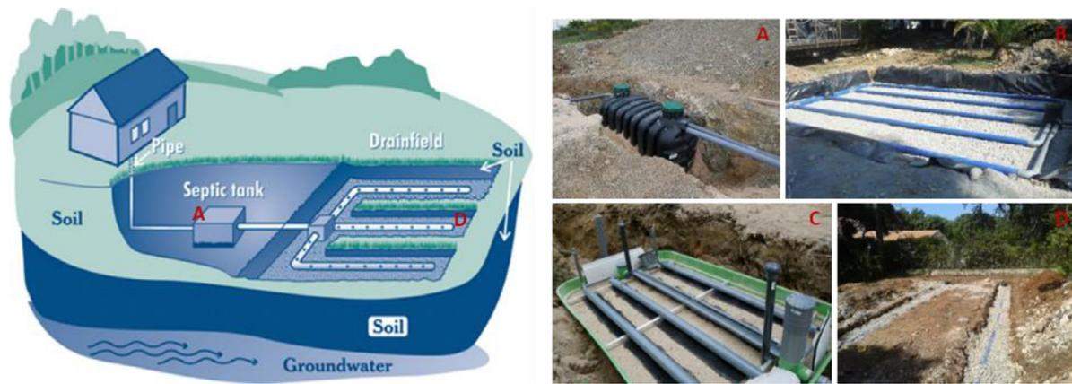
Fig. 1. Schematic representation of a septic system (adapted from EPA (2005)) and illustrative photos before filling operation (© KD, A: septic tank, B: sand filter, C: media filter, D: drain field).
