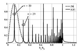
**FIGURE 11.** Comparison of the normalized Hankel transform of the BGB field distribution (dashed line) and the magnitude of the spectral Green's function component  $G_{\phi\phi}^{HM}$  (solid line) at z=0,  $L=14.7\lambda$ ,  $f_0=2.5$  GHz.  $k_\rho/k_0$  represents the spectral wavenumber normalized to the wavenumber in free space.
