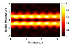
FIGURE 9. Normalized simulated amplitudes of the E-field of the BGB launcher in the x0z plane between two apertures when  $L=3.15\lambda$ .
