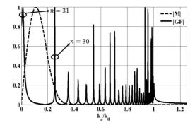
FIGURE 12. Comparison of the normalized Hankel transform of the BGB field distribution (dashed line) and the magnitude of the spectral Green's function component  $G_{\phi\phi}^{HM}$  (solid line) at z=0,  $L=14.7\lambda$ ,  $f_0=2.565$  GHz.  $k_\rho/k_0$  represents the spectral wavenumber normalized to the wavenumber in free space.
