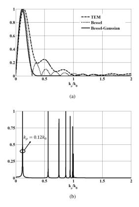
FIGURE 5. (a) Normalized Hankel transform of TEM (dashed line), BB (dotted line), and BGB (solid line) field distributions.  $k_\rho/k_0$  represents the spectral wavenumber normalized to the free space wavenumber. (b) Magnitude of the spectral Green's function component  $G_{\phi\phi}^{HM}$  of the equivalent PPW at z=0 when  $L=2.94\lambda$ .
