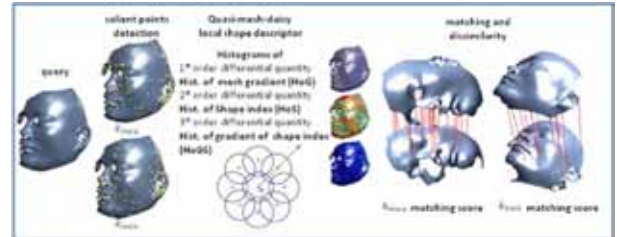
Quasi-mesh-daisy local shape descriptor based free-form surface matching framework.
