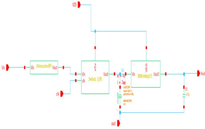
Fig. 1. Schematic of the S&H voltage sensor.
