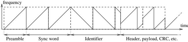
Fig. 1: Example of a partial LoRa frame.
