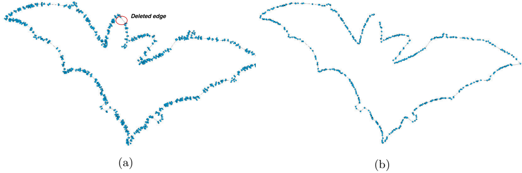
Figure 1: (a) A geometric graph representing a bat's shape. (b) The approximated longest path found after breaking the cycle by removing one edge.
