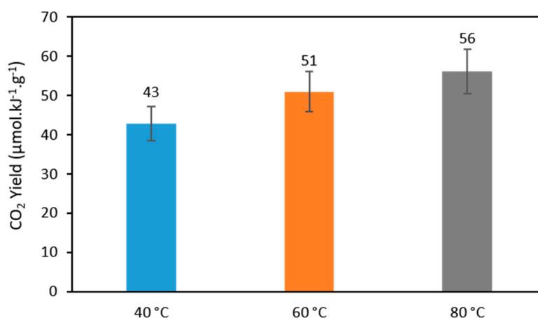
**Figure 9.** Calculated CO<sub>2</sub> yield from the photothermal treatment of 0.01 mM RhB solutions in the presence of Ti@TiO<sub>2</sub> photocatalyst under Ar/20% O<sub>2</sub> atmosphere at 40, 60 and 80 °C (catalyst concentration 0.12 g<sup>-1</sup>.L<sup>-1</sup> V = 60 mL, P<sub>Xe light</sub> = 9.5 W). Emission profiles of CO<sub>2</sub> emission are shown in Figure S14.
