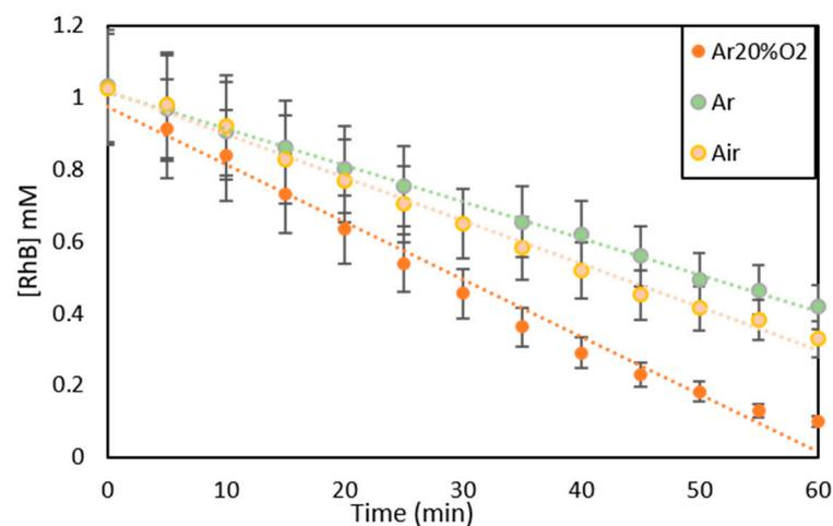
**Figure 7.** Kinetics of RhB evolution upon sonolysis of RhB with 345 kHz US in the absence of any solid particles under different gas atmospheres ( $V_{\text{RhB}} = 200 \text{ mL}$ ,  $T = 40 \text{ }^\circ\text{C}$ ).
