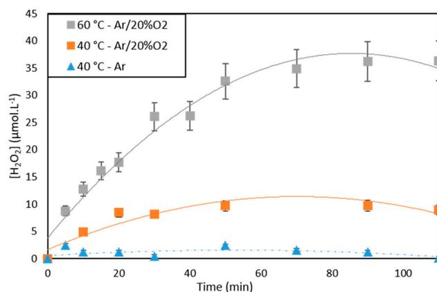
**Figure 5.**  $H_2O_2$  concentration produced during photocatalytic experiments with 0.02 M  $TiOSO_4/0.25$  M  $H_2SO_4$  solutions over  $Ti@TiO_2$  NPs at different temperatures (catalyst concentration  $2$  g  $L^{-1}$ ,  $V = 65$  mL). Concentration of  $TiO(O_2)$  complex equal to that of formed  $H_2O_2$  was monitored at 410 nm ( $\epsilon = 626$   $cm^{-1} \cdot M^{-1}$ ) [26].
