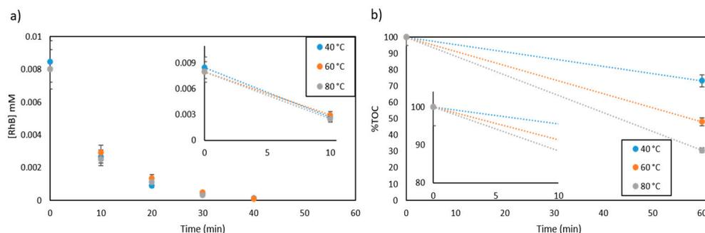
**Figure 8.** Kinetic curves of 0.01 mM RhB degradation and (a) TOC removal (b) in the presence of Ti@TiO<sub>2</sub> NPs under Ar/20% O<sub>2</sub> flux at three different temperatures. Catalyst concentration  $0.12 \text{ g}^{-1}\cdot\text{L}^{-1}$ .
