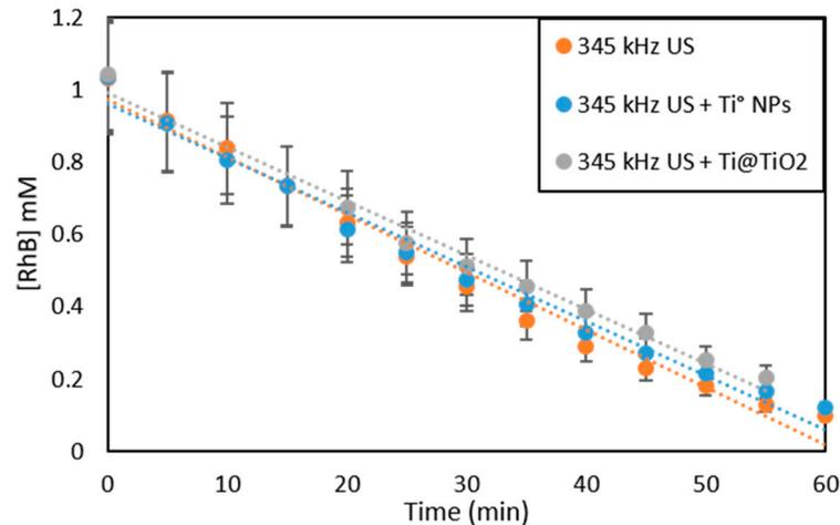
**Figure 6.** Kinetic curves of RhB evolution upon sonolysis of homogeneous RhB solution and sonochemical oxidation of RhB in the presence of  $\text{Ti}^0$  and  $\text{Ti@TiO}_2$  NPs in Ar/20%  $\text{O}_2$  at (catalyst concentration  $2 \text{ g L}^{-1}$ ,  $T = 40 \text{ }^\circ\text{C}$ ).
