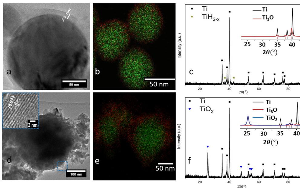
**Figure 1.** TEM images, STEM/EDX mapping and XRD diffraction patterns of air passivated Ti<sup>0</sup> NPs (a–c) and Ti@TiO<sub>2</sub> NPs (d–f). Green dots—Ti, red dots—O.
