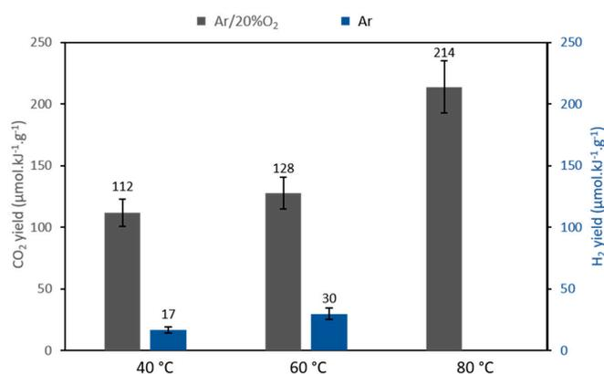
**Figure 3.** Yields of CO<sub>2</sub> for Ar/20% O<sub>2</sub> atmosphere (grey) and H<sub>2</sub> for Ar atmosphere (blue) yields obtained upon photocatalytic degradation of 5 mM EDTA solution over Ti@TiO<sub>2</sub> catalyst under Ar/20% O<sub>2</sub> and Ar at different temperatures (catalyst concentration 0.12 g·L<sup>-1</sup>, V = 65 mL, P<sub>Xe</sub> = 9.5 W).
