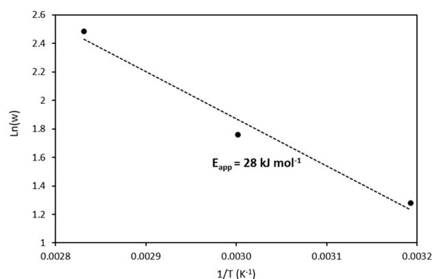
**Figure 4.** Arrhenius plot for the photocatalytic EDTA degradation in the presence of Ti@TiO<sub>2</sub> NPs under Ar/O<sub>2</sub> atmosphere, W is an EDTA degradation rate assuming zero-order kinetics.
