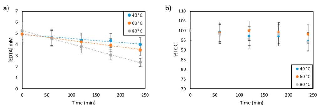
**Figure 2.** Kinetic curves of EDTA evolution and (a) TOC abatement curves (b) during photolysis of 5 mM initial EDTA solutions under  $\text{Ar}/20\% \text{O}_2$  atmosphere at 3 different temperatures in the presence of  $\text{Ti@TiO}_2$  NPs (catalyst concentration  $0.12 \text{ g}\cdot\text{L}^{-1}$ ,  $V = 65 \text{ mL}$ ,  $P_{\text{light}} = 9.5 \text{ W}$ ).
