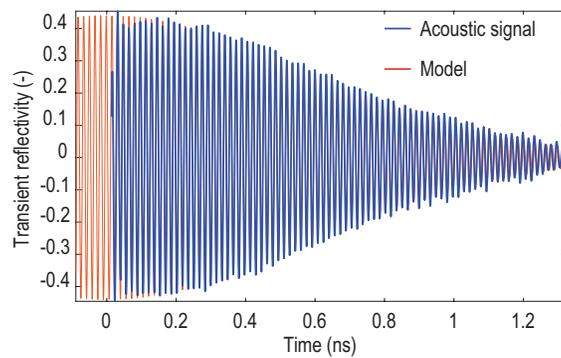
Figure 8: Comparison between the acoustic contribution to the transient reflectivity signal measured by the photodiode, located at the position  $x = 25.79 \mu\text{m}$  and  $y = 23.45 \mu\text{m}$  of the scan, and the Gaussian damping model signal obtained by fitting. (colors needed)
