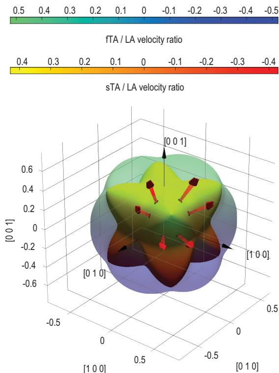
Figure 6: 3-D surfaces of shear velocity ratio to LA. The fTA/LA velocity ratio surface is transparent for better visualization of the sTA/LA one. The possible orientations of the grain 1A, in which the 3 acoustic quasi-modes are monitored, are represented by red arrows (with black circle basis) in 1/8 of the surface. Due to symmetries in the cubic crystalline structure, 6 orientations with common velocity ratio are obtained. (colors needed)
