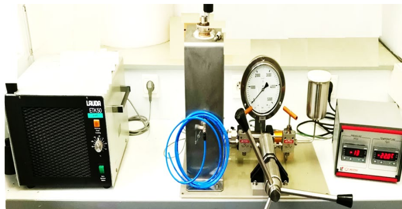
Figure 2. Freeze isostatic pressure equipment at ICMCB.
