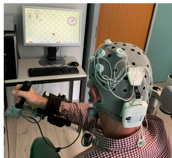
Fig. 4 Anodal HD-tDCS applied to the ipsilesional primary motor cortex during an ARMEO virtual reality therapy session using the right upper limb. The patient is setup on the ARMEO exoskeleton equipped with the HD-tDCS cap comprising a Starstim NIC-power box delivering the current on the back and 5 electrodes located on the left primary motor cortex in a 4x1 HD-tDCS montage with anode on the C3 location
