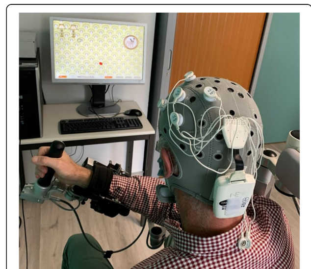
Fig. 4 Anodal HD-tDCS applied to the ipsilesional primary motor cortex during an ARMEO virtual reality therapy session using the right upper limb. The patient is setup on the ARMEO exoskeleton equipped with the HD-tDCS cap comprising a Starstim NIC-power box delivering the current on the back and 5 electrodes located on the left primary motor cortex in a 4x1 HD-tDCS montage with anode on the C3 location
