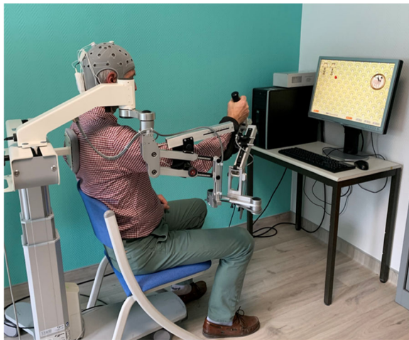
Fig. 2 Patient setup on the ARMEO virtual reality therapy system. The ARMEO exoskeleton counterbalances the weight of the patient's upper limb with springs located on the elbow and wrist joints. The patient in a resting position, ready to begin to play the ladybug game
