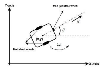
Fig. 1. Schematic diagram of differential drive robot
