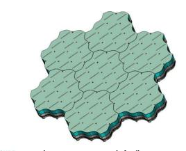
FIGURE 23. 84 elements array composed of 7 tiles.
