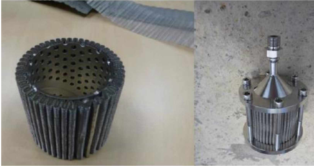
Fig. 3: cartridge section (52 mm length) of the MF (left) equipped with flanges for irradiation (right)
