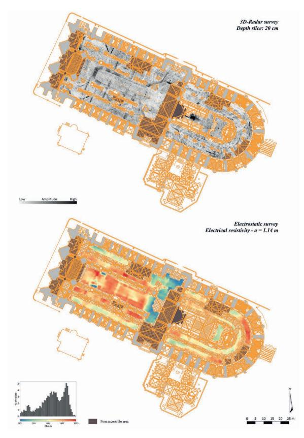
Figure 3. 3D-Radar and electrostatic maps (CAD: AGP/Inrap).
