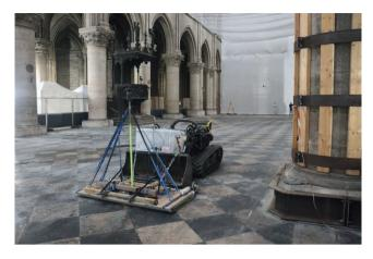
Figure 1. 3D-Radar survey with remote-controlled machine in the nave.
