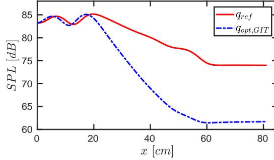
Figure 15: Sound pressure levels measured along the top wall (see Fig. 4) for the input plane wave packet centred around 1500Hz. The TDIBC is located at the bottom wall, between  $20.3cm \leq x \leq 60.9cm$ .
