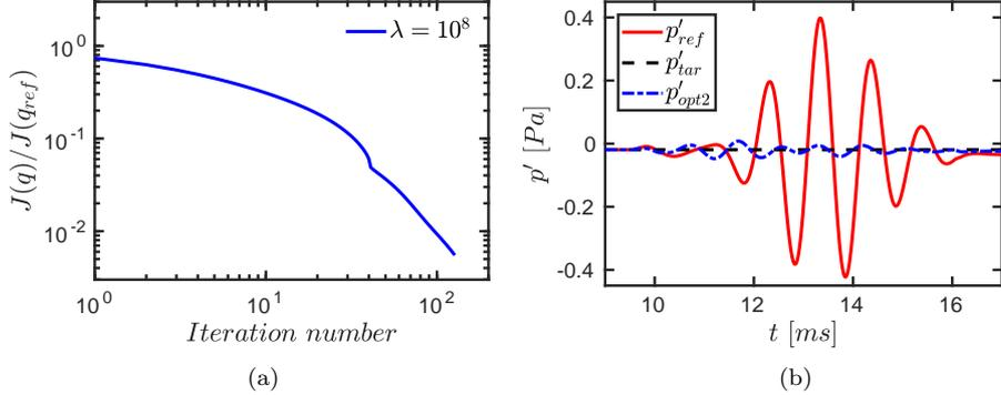
Figure 7: Optimization at constant  $\tau$  and  $\beta_\infty$ . (a) Convergence of  $J(q)$  towards a minimum value during the gradient descent optimization. For  $\lambda = 10^8$ ,  $J(q)/J(q_{ref})$  reaches 0.55% before the descent algorithm starts oscillating. We take  $q_{opt2}$  to be  $q$  recovered after 128 iterations. (b) Reflected pressure perturbations (reference and optimized), and target perturbation level  $p'_{tar}$ .
