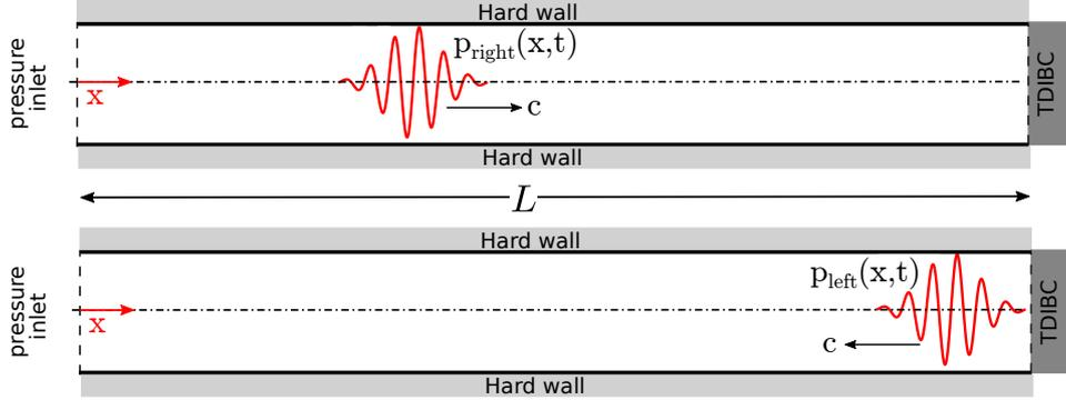
Figure 1: Sketch of the 1D impedance tube test case. The inlet packet of pressure fluctuations travels towards positive  $x$  at the sound speed  $c$  (top). At  $x = L = 1.8$  m, a TDIBC is located which interacts with the incident wave packet, reflecting it back towards the inlet (bottom).
