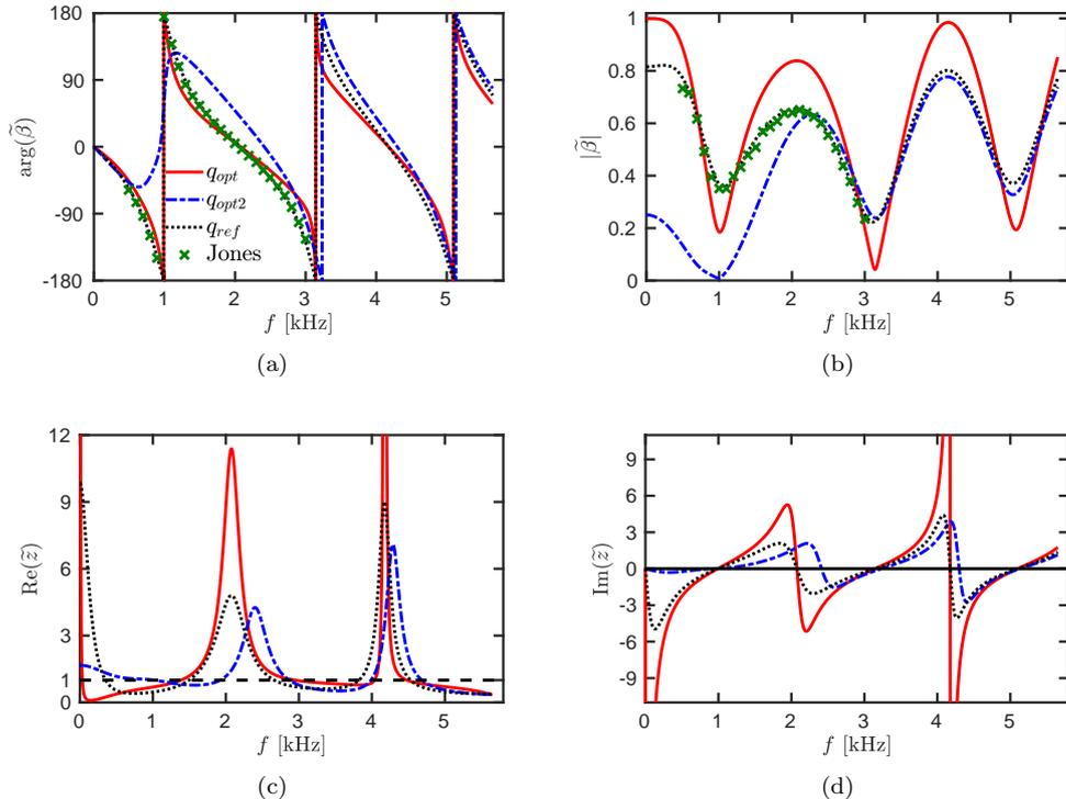
Figure 6: (a) Argument and (b) modulus of the reflection coefficient  $\tilde{\beta}(s)$  based on  $q_{ref}$ ,  $q_{opt}$  and  $q_{opt2}$  in Table 1. (c) Real and (d) imaginary part of the impedance  $\tilde{z}(s)$  based on  $q_{ref}$ ,  $q_{opt}$  and  $q_{opt2}$ .  $\tilde{z} = (1 + \tilde{\beta})/(1 - \tilde{\beta})$ .
