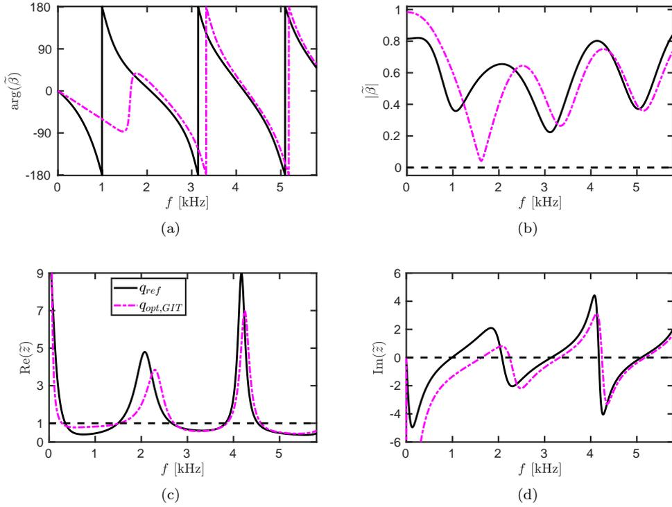
Figure 16: (a) Argument and (b) modulus of the reflection coefficient  $\tilde{\beta}(s)$  based on  $q_{ref}$  and  $q_{opt,GIT}$ . (c) Real and (d) imaginary part of the impedance  $\tilde{z}(s)$ .  $\tilde{z} = (1 + \tilde{\beta})/(1 - \tilde{\beta})$ .
