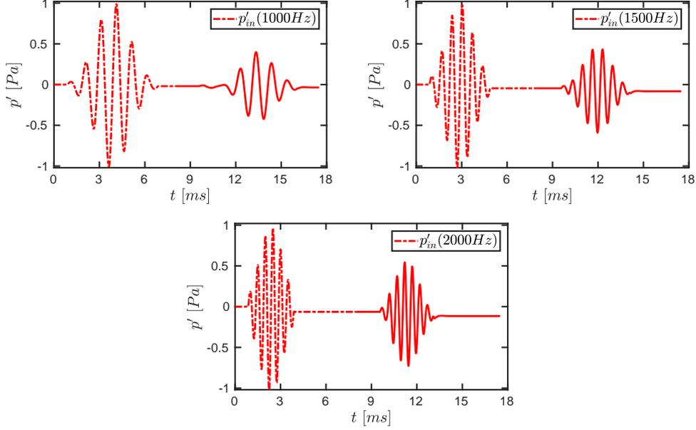
Figure 8: Pressure perturbations  $p'$  measured about the ambient value  $p_a = 101325$  Pa at the probe location  $x = 0.3$  m in the 1D impedance tube. Dashed lines correspond to the right-running wave packet coming from the inlet, while the solid portion corresponds to the perturbations reflected by the TDIBC operating with parameters set at  $q_{ref}$  – see Table 1.
