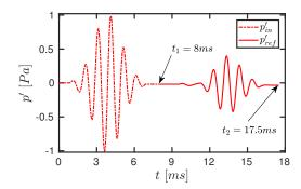
Figure 3: Pressure perturbations p' measured about the ambient value  $p_a=101325$  Pa at the probe location x=0.3 m. The oscillations for  $t< t_1$  are due to the incident wave packet characterized in Fig. 2 travelling from the inlet at x=0 towards the TDIBC wall at x=1.8 m. The interval between  $t_1$  and  $t_2$  is chosen to study the properties of the pressure perturbations reflected by the TDIBC back towards the inlet.
