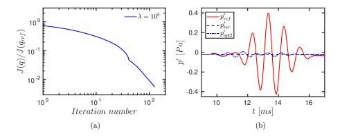
Figure 7: Optimization at constant  $\tau$  and  $\beta_{\infty}$ . (a) Convergence of J(q) towards a minimum value during the gradient descent optimization. For  $\lambda=10^8$ ,  $J(q)/J(q_{ref})$  reaches 0.55% before the descent algorithm starts oscillating. We take  $q_{opt2}$  to be q recovered after 128 iterations. (b) Reflected pressure perturbations (reference and optimized), and target perturbation level  $p'_{tar}$ .
