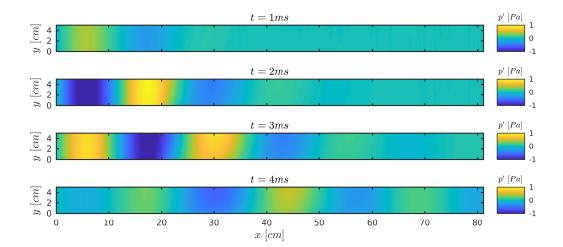
Figure 12: Plane wave packet evolution in the GIT test case, travelling at the speed of sound c=344.37~m/s towards the right. The TDIBC is located at the bottom wall, between 20.3 cm  $\leq x \leq 60.9~\text{cm}$  – see Fig. 4. Simulation results obtained with the TDIBC parameters before optimization –  $q_{ref}$  shown in Table 1.
