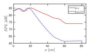
Figure 15: Sound pressure levels measured along the top wall (see Fig. 4) for the input plane wave packet centred around 1500Hz. The TDIBC is located at the bottom wall, between  $20.3cm \le x \le 60.9cm$ .
