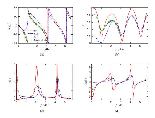
Figure 6: (a) Argument and (b) modulus of the reflection coefficient  $\widetilde{\beta}(s)$  based on  $q_{ref}$ ,  $q_{opt}$  and  $q_{opt2}$  in Table 1. (c) Real and (d) imaginary part of the impedance  $\widetilde{z}(s)$  based on  $q_{ref}$ ,  $q_{opt}$  and  $q_{opt2}$ .  $\widetilde{z} = (1 + \widetilde{\beta})/(1 - \widetilde{\beta})$ .
