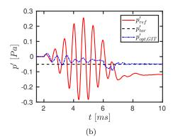
Figure 14: (a) Convergence of J(q) towards a minimum value during the gradient descent optimization. For  $\lambda=100,\ J(q)/J(q_{ref})$  reaches 6.9% while for  $\lambda=1000,\ J(q)/J(q_{ref})$  reaches 8%. In both cases, the optimization is terminated due to the  $|\widetilde{\beta}(s)| \leq 1$  condition being violated at 0Hz. (b) Pressure fluctuations (reference and optimized) at the probe location  $(x=70cm,\ y=5cm)$  for the 2D GIT case, and target pressure level  $p'_{tar}$ .
