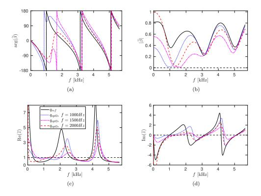
Figure 10: (a) Argument and (b) modulus of the reflection coefficient  $\widetilde{\beta}(s)$  based on  $q_{ref}$  and  $q_{opt3}$  for the three analysed frequencies f. (c) Real and (d) imaginary part of the impedance  $\widetilde{z}(s)$ .  $\widetilde{z} = (1+\widetilde{\beta})/(1-\widetilde{\beta})$ .
