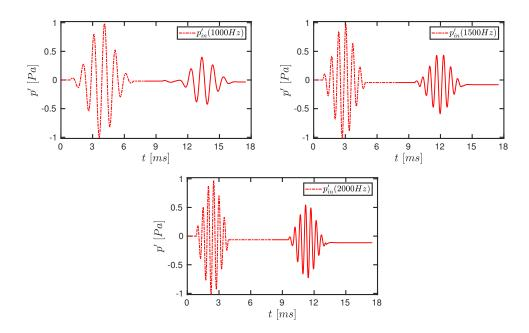
Figure 8: Pressure perturbations p' measured about the ambient value  $p_a=101325$  Pa at the probe location x=0.3 m in the 1D impedance tube. Dashed lines correspond to the right-running wave packet coming from the inlet, while the solid portion corresponds to the perturbations reflected by the TDIBC operating with parameters set at  $q_{ref}$  – see Table 1.
