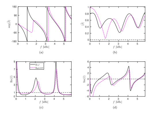
Figure 16: (a) Argument and (b) modulus of the reflection coefficient  $\widetilde{\beta}(s)$  based on  $q_{ref}$  and  $q_{opt,GIT}$ . (c) Real and (d) imaginary part of the impedance  $\widetilde{z}(s)$ .  $\widetilde{z} = (1 + \widetilde{\beta})/(1 - \widetilde{\beta})$ .
