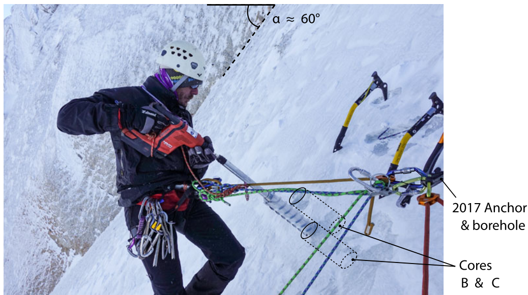
Fig. 3. Coring in the north face of TDT. Core A was drilled where the photographer stands.
