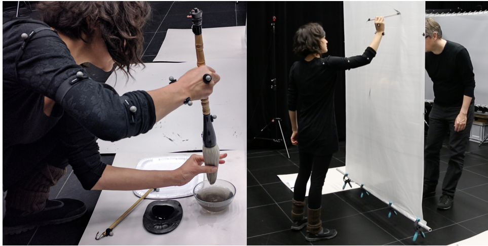
Figure 1: Marker placement on arm, hand & brushes (left) and two-person performance with motion capture (right).
