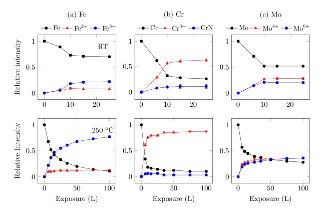
Figure 7: Evolution of (a) iron, (b) chromium and (c) molybdenum at RT (top) between 0-25 L, and 250 °C (bottom) between 0-100 L oxygen exposure at a  $45^{\circ}$  take-off angle.
