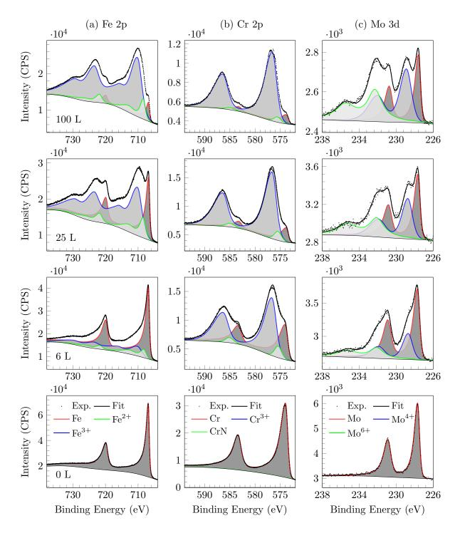
Figure 2: High resolution XPS spectra of (a) iron, (b) chromium and (c) molybdenum recorded after oxygen exposures of 0, 6, 25 and 100 L at 250  $^{\circ}$ C.
