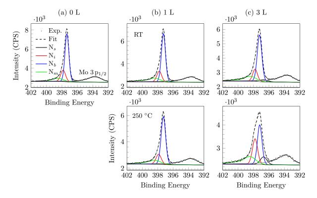
Figure 5: High resolution XPS spectra of the N 1s region during the first 3 L of oxygen exposure at both RT (top) and 250 °C (bottom), showing the four identified components,  $N_s$  (surface nitride),  $N_i$  (interstitial nitrogen),  $N_b$  (bulk nitride) and  $N_m$  (minority nitrogen).
