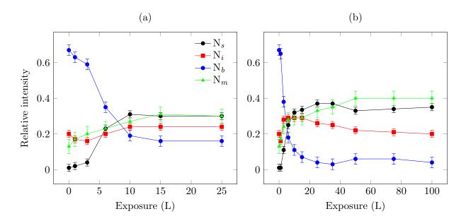
Figure 6: Evolution of relative nitrogen component intensities as a function of oxygen exposure at (a) RT and (b) 250 °C.
