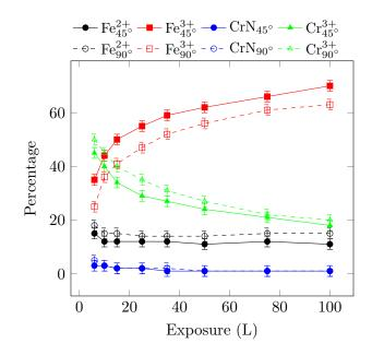
Figure 9: Composition of oxide film at 250  $^{\circ}$ C as a function of oxygen exposure at 45 $^{\circ}$  and 90 $^{\circ}$  photoelectron take-angles.
