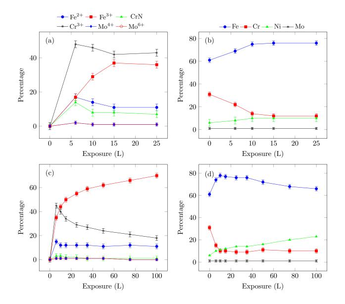
Figure 8: Composition of the (a) oxide at RT, (b) modified alloy at RT, (c) oxide at 250  $^{\circ}$ C, and (d) modified alloy at 250  $^{\circ}$ C, as a function of oxygen exposure.
