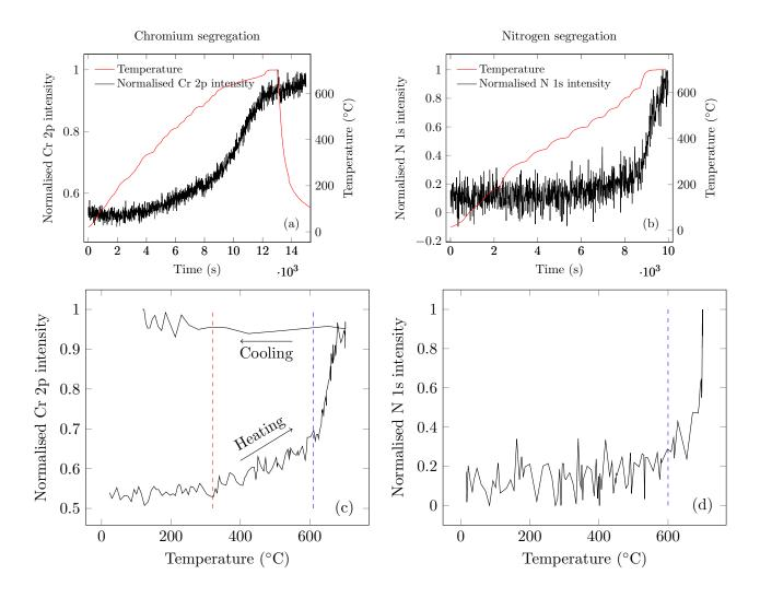
Figure 1: Real-time segregation of elements during the annealing process as measured using XPS snapshot measurements: (a) variation of normalised Cr 2p intensity, (b) variation of normalised N 1s intensity, (c) Normalised Cr 2p intensity as a function of annealing temperature, (d) Normalised N 1s intensity as a function of annealing temperature.
