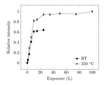
Figure 4: Relative intensity of O 1s signal plotted as a function of oxygen exposure at both RT and 250 °C.
