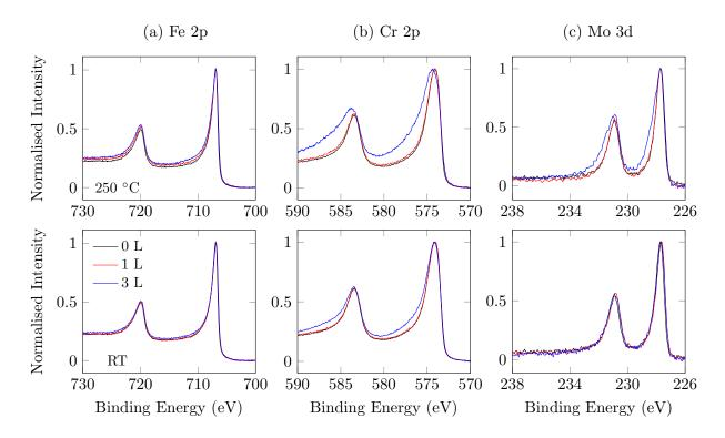
Figure 3: Comparison of peak shapes for (a) Fe 2p, (b) Cr 2p and (c) Mo 3d during the first 3 L of oxygen exposure at RT (top) and 250 °C (bottom).
