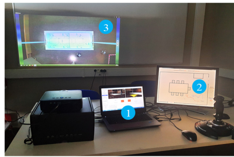
Figure 5. Logistics workplace (Organization 2). (1) Logistics control interface; (2) Tactical interface; (3) Bird's eye view of the production cell.
