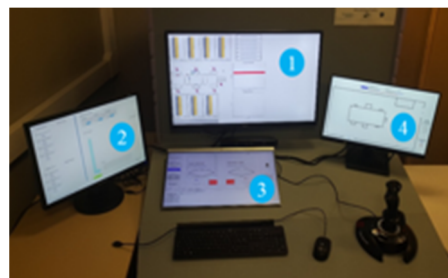
Figure 3. Workplace to control the intelligent manufacturing system (Organization 1). (1) Production control interface; (2) Planning interface; (3) Logistics control interface; (4) Tactical interface.
