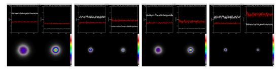
Fig. 2. Strehl and FWHM, White, no correction; red, correction; from left to right:  $\lambda = 500$ nm,  $r_0=7$ cm and  $r_0=20$ cm;  $\lambda = 700$ nm,  $r_0=7$ cm,  $r_0=20$ cm. In all cases the wavefront sensor has  $11 \times 11$  subapertures, collecting  $2 \times 10^5$  photons per integration (at 500Hz) over a 30' field of view. Lower row shows corrected and uncorrected PSFs on same scale.
