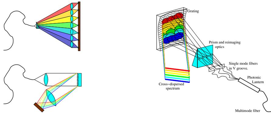
**Fig. 2. Left:** Conceptual spectrograph using a prism (left) or grating/VPH (right), fed by a multi-mode fiber. Although simple in design, the main issue with such concepts are the size and the stability. **Right:** Using a photonic lantern and a V-groove to align the single mode fibers into a pseudo slit, a single mode, bulk optics spectrograph can be used, allowing for a more compact design.
