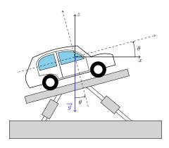
Fig. 1. Driving simulator scheme
