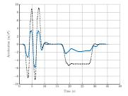
Fig. 5. Acceleration reference profile (dashed), output acceleration (blue)
