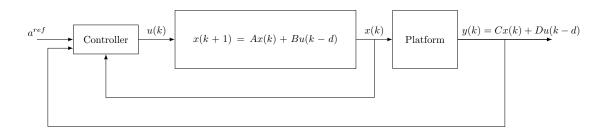
Fig. 2. Block diagram of the control structure operating
