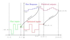
Fig. 3. Principle of the strategy proposed in Section III, the past inputs impose the free response up to k+d while the optimized inputs are chosen such that the predicted inputs ensure the first predicted state (at stage k+d+1) to belong to the controllable set  $\mathcal C$
