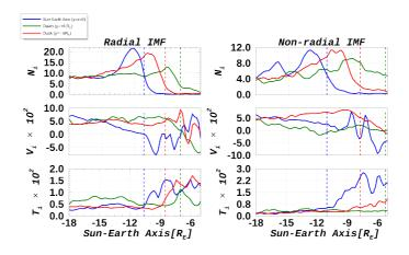
Figure 11. Ion density, velocity, and temperature  $(N_i, V_i, T_i)$  are plotted along the OX-axis and at  $\pm 6$  on both dusk and dawn directions in the XY plane. Vertical dashed lines show the MP position at the subsolar point(blue), dusk flank(red), and dawn flank(green) quantities show dusk-dawn asymmetry at the  $\pm 6R_E$ .
