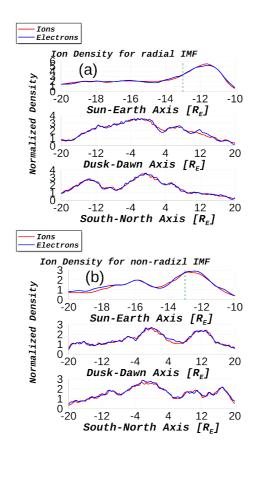
Figure 8. Ion and electron densities are plotted in three directions, along OX (Y=Z=0), OY (X=-13, and Z=0), and OZ (X=-13, and Y=0)), just outside the MP for radial IMF in panel a and for non-radial IMF in panel b. Their values are normalized to the initial densities. The density profile is plotted only in the dayside region as shown with vertical dashed lines (at  $X = -13R_E$ ) in Fig. 2. This figure also shows the plasma quasi neutrality.
