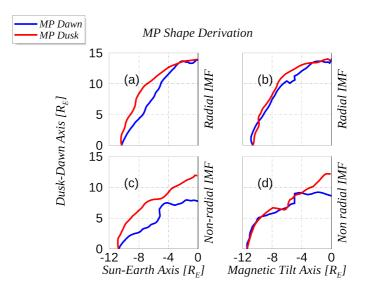
Figure 7. Panels (a) and (b) show the MP shape for radial IMF along Sun-Earth and tilted magnetic equatorial axis. Similarly, panels (c) and (d) are the same but for non-radial IMF. We remark that the size shown here is approximately equivalent to the MP sizes derived from the density steepening.
