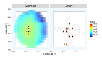
Fig. 1 MRFS-MI and mRMR score-based maps obtained considering a 1-hour forecasting horizon. Black dots stand for the position of the 10 most informative features while the grey dot represents the site location.
