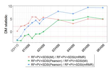
Fig. 3 DM statistic between the three SDSI feature selection frameworks studied for different forecast horizons. The red dotted lines stand for the borders delimiting the validation and rejection of the null hypothesis.
