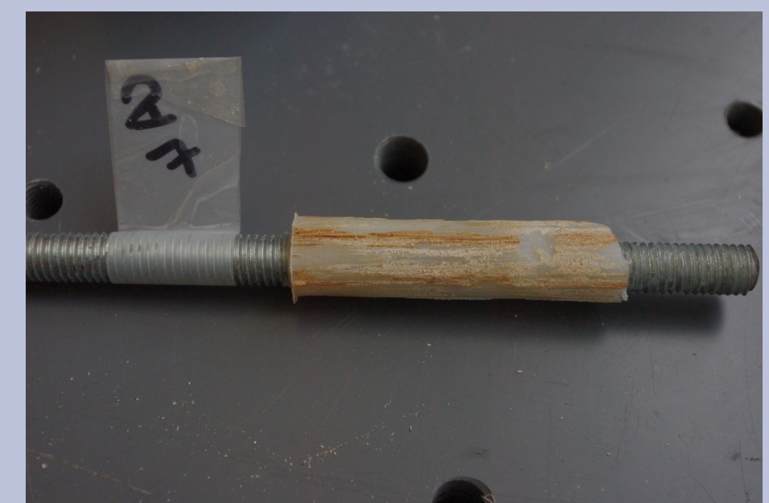
Failure at timber/glue interface
