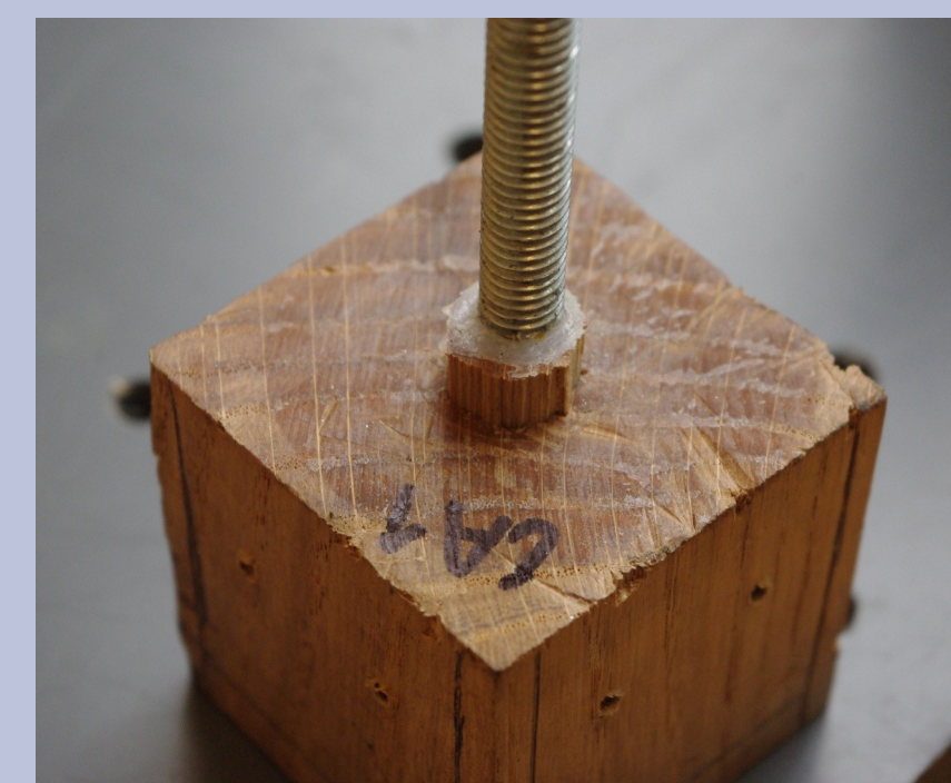
Failure at timber/glue interface
