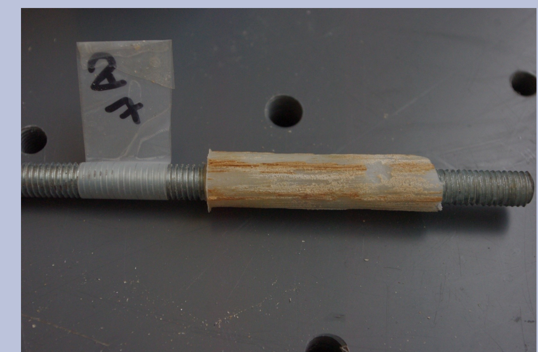
Failure at timber/glue interface
