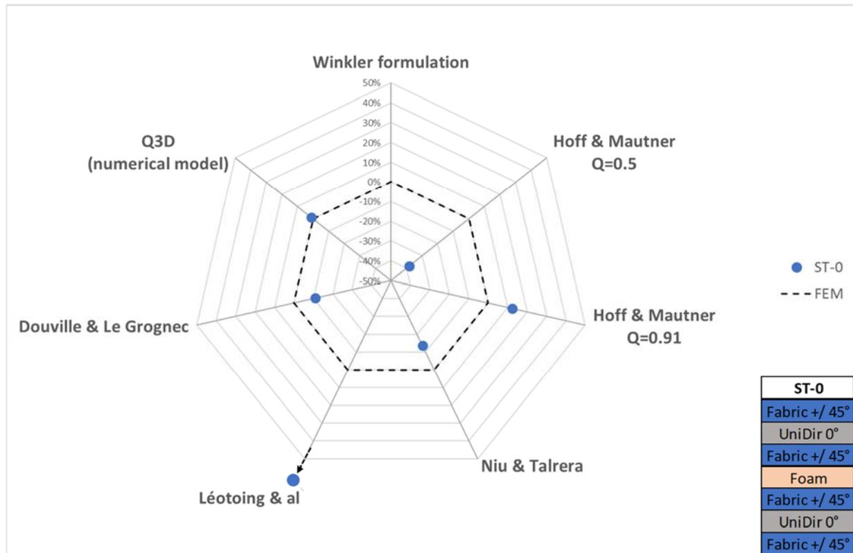
Figure 8: Radar type comparison graph for ST-0 sandwich stacking: symmetric balanced orthotropic skin with foam core.
