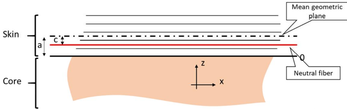
Figure 6: Definition of the asymmetry parameter  $\varphi$
