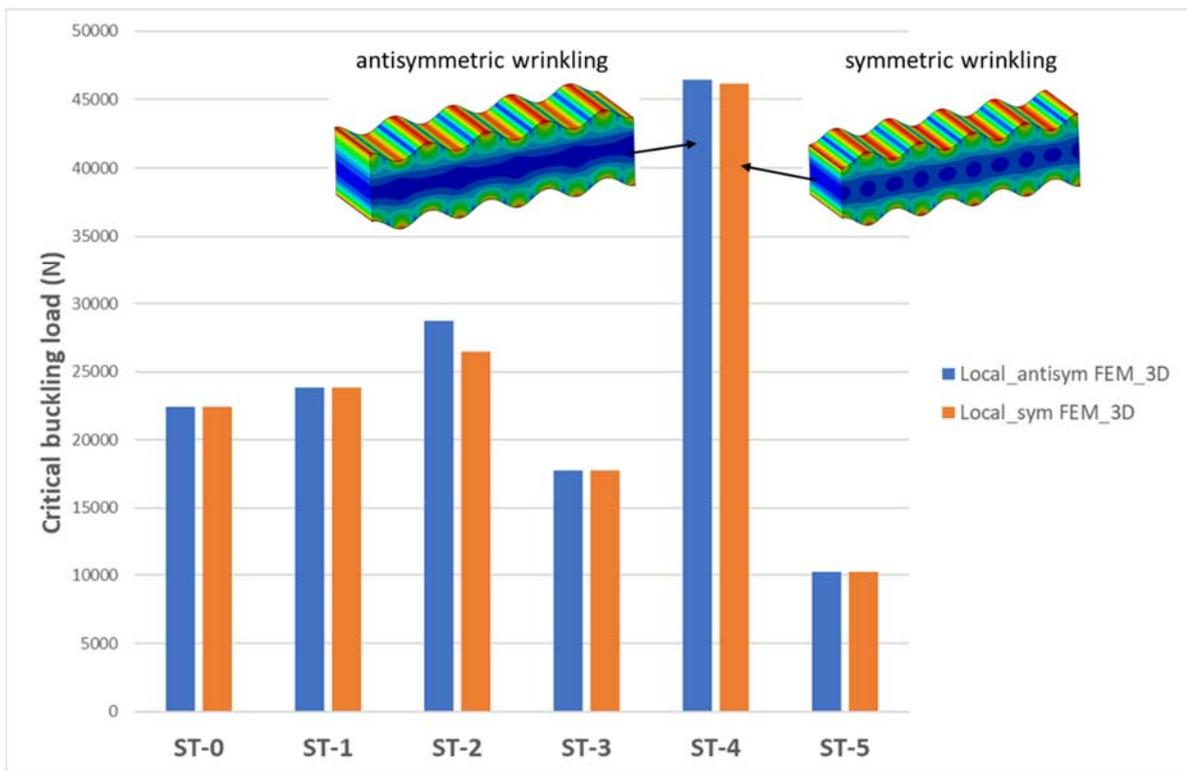
Figure 7: 3D FEM critical local buckling load for antisymmetric and symmetric modes
