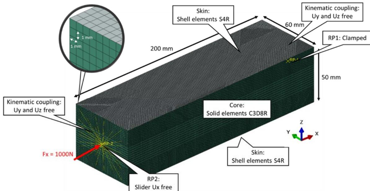
Figure 4: 3D FEM with its boundary conditions
