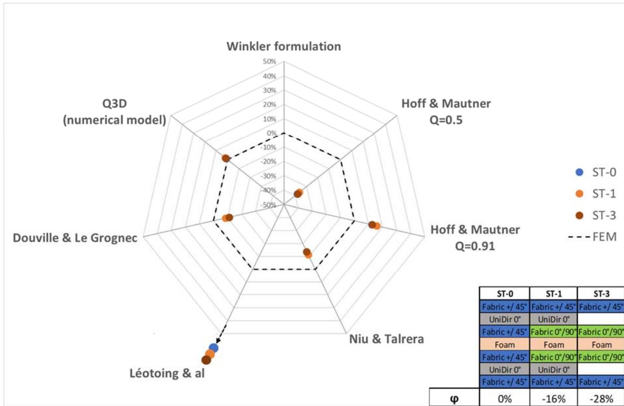
Figure 10: Radar type comparison graph for symmetric skins (ST-0) and asymmetric skin (ST-1; ST-3)
