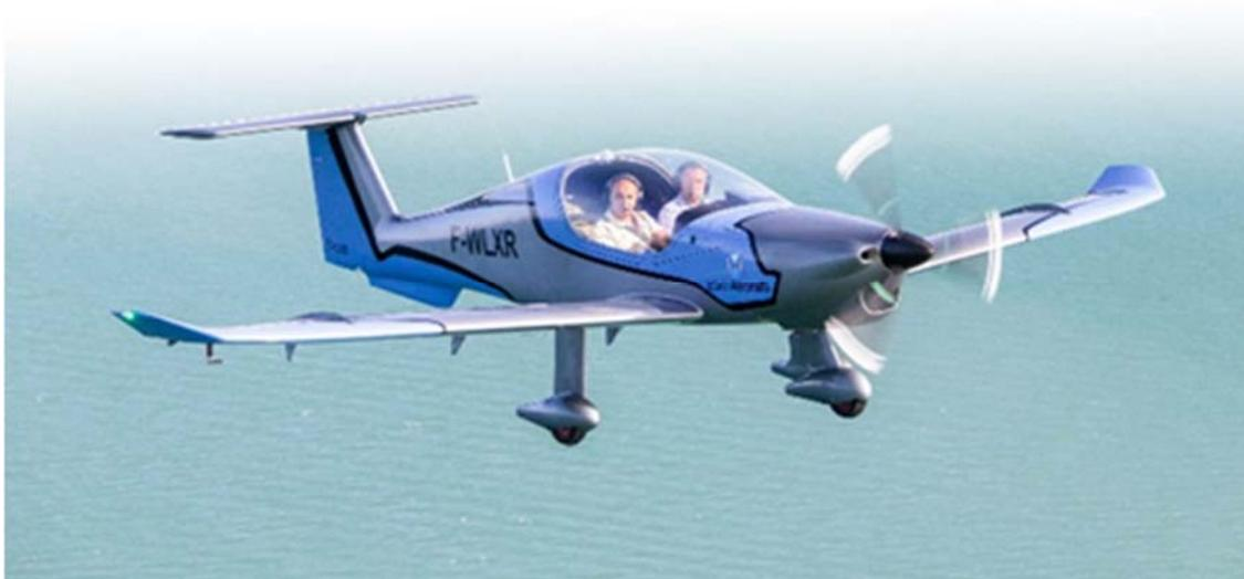
Figure 1: The Elixir, EASA certified two-seater light aircraft (<https://elixir-aircraft.com>).
