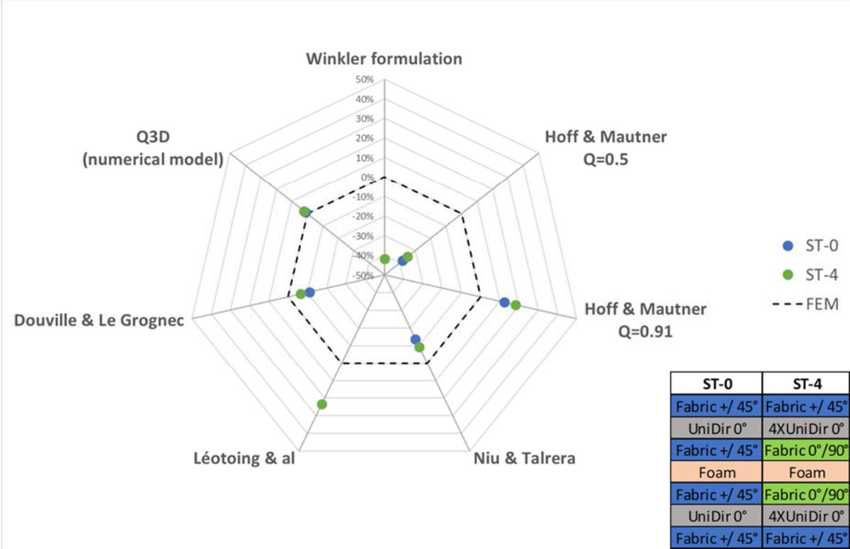
Figure 11: Radar type comparison graph for ST-0 and ST-4 with a large proportion of UniDirectional ply
