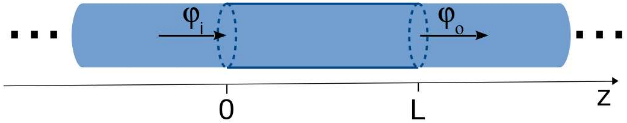
FIG. 3: Schematics of the NW of finite length L periodised along z . \varphi_i and \varphi_o are the inward and outward thermal currents.
