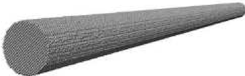
FIG. 1: Atomic structure of a crystalline silicon nanowire with D=10 nm and L=200 nm.
