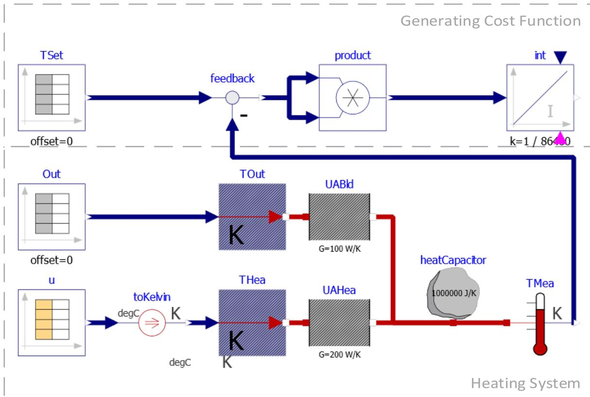
**Figure 1.** Residential heating system developed in OpenModelica
