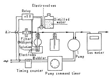
Fig. 3. Schema of  $SO_2$  sampling device.
