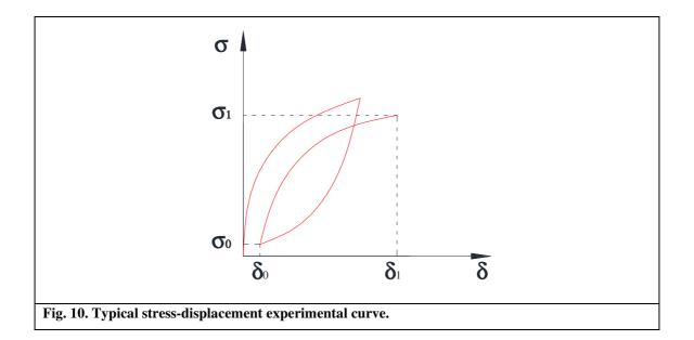
The symbol K<sub>exp</sub> indicates the experimental stiffness of the adhesive, evaluated over the generic step
