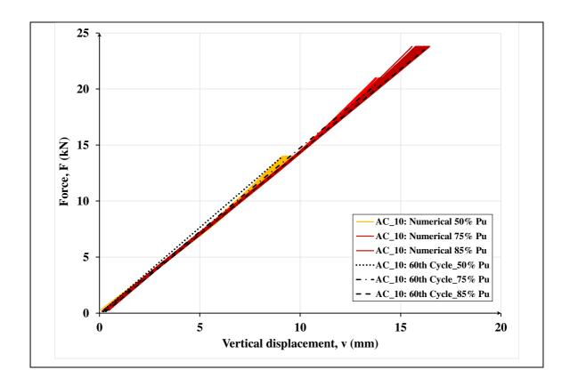
Fig. 22. Comparison of computed and experimental force-displacement curve for GFRP hollow column to built-up beam adhesive connection (test denoted AC\_10).
