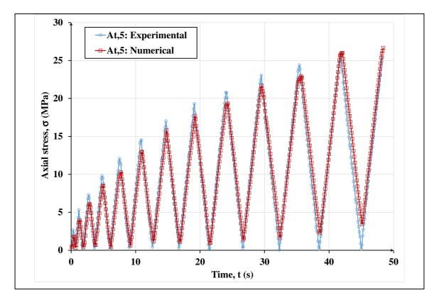
Fig. 14. Comparison of computed and experimental stress-time curve for adhesive of 5 mm thickness (At,5).
