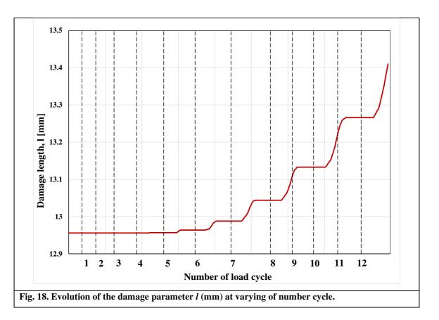
15 Finally, the graph depicted in Fig. 18 permitted to conclude that the evolution of the damage parameter *l* is strongly non-linear when an adhesive layer is subject to variable actions. 16
