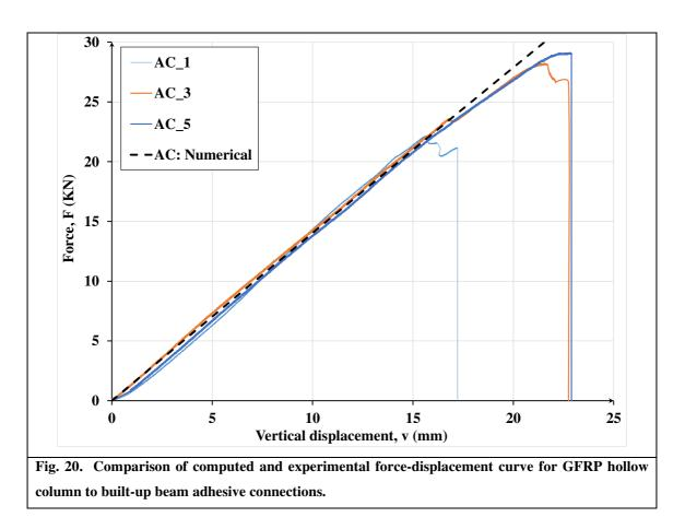
Furthermore, the comparison of computed and experimental force-displacement curve for GFRP
